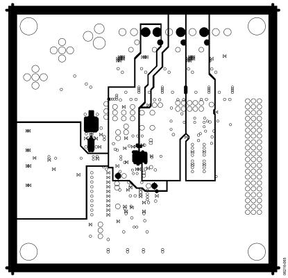
Figure 61. Evaluation Board Layout, Power Plane
