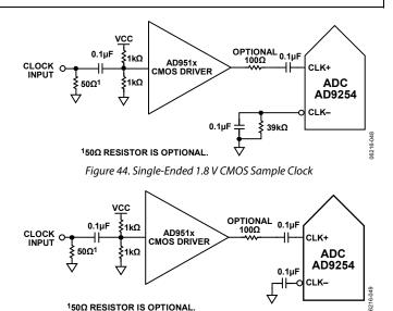
Figure 45. Single-Ended 3.3 V CMOS Sample Clock
