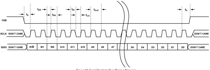
Figure 50. Serial Port Interface Timing Diagram
