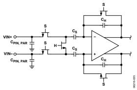
Figure 31. Switched-Capacitor SHA Input
