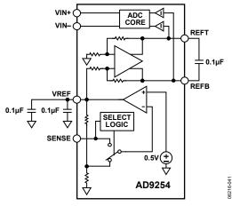
Figure 37. Internal Reference Configuration
