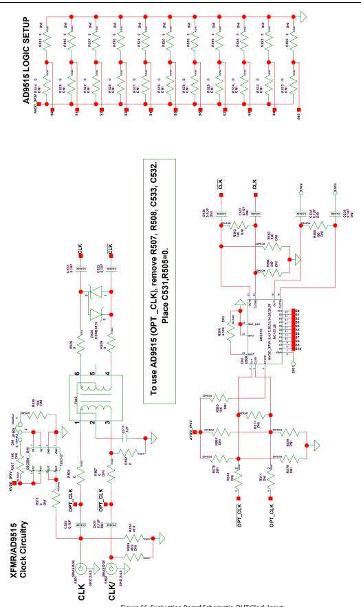
Figure 55. Evaluation Board Schematic, DUT Clock Input
