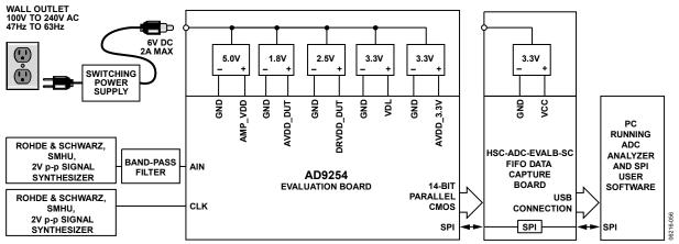
Figure 52. Evaluation Board Connection
