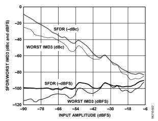
Figure 22. AD9254 Two-Tone SFDR/IMD3 vs. Input Amplitude (AIN) with  $f_{\rm IN1}$  = 29.1 MHz,  $f_{\rm IN2}$  = 32.1 MHz
