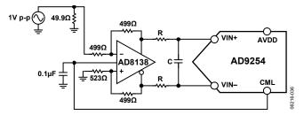
Figure 32. Differential Input Configuration Using the AD8138
