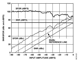
Figure 21. AD9254 Single-Tone SNR/SFDR vs. Input Amplitude (AIN) with  $f_{\rm IN}$  = 2.4 MHz
