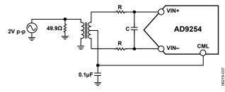
Figure 33. Differential Transformer-Coupled Configuration
