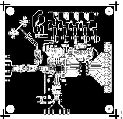
Figure 58. Evaluation Board Layout, Primary Side
