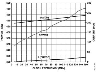
Figure 47. AD9254 Power and Current vs. Clock Frequency  $f_{IN} = 30 \text{ MHz}$
