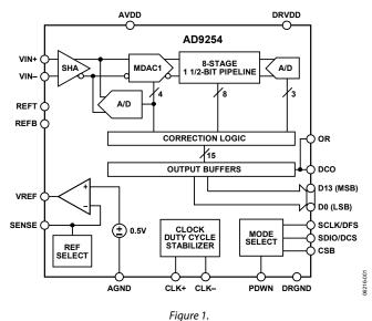
The digital output data is presented in offset binary, Gray code, or twos complement formats. A data output clock (DCO) is provided to ensure proper latch timing with receiving logic.
