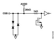
Figure 9. Equivalent CSB Input Circuit
