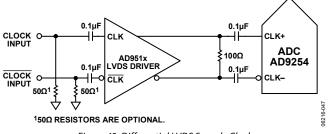
Figure 43. Differential LVDS Sample Clock
