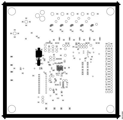
Figure 60. Evaluation Board Layout, Ground Plane
