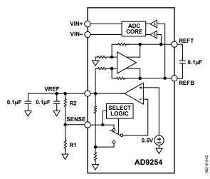
Figure 38. Programmable Reference Configuration
