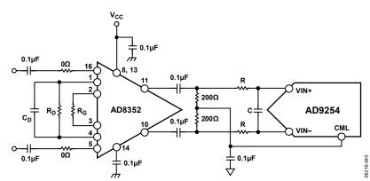
Figure 36. Differential Input Configuration Using the AD8352
