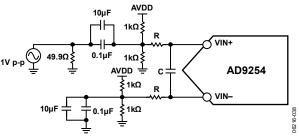
Figure 34. Single-Ended Input Configuration
