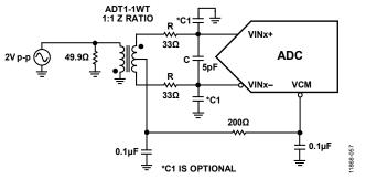
Figure 50. Differential Transformer-Coupled Configuration for Baseband Applications
