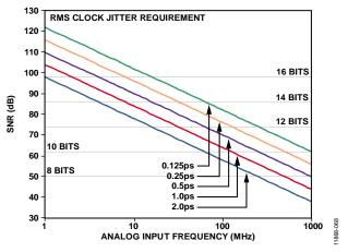
Figure 62. Ideal SNR vs. Analog Input Frequency and Jitter
