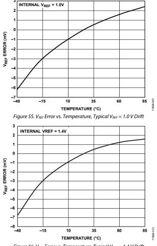
Figure 56.  $V_{REF}$  Error vs. Temperature, Typical  $V_{REF} = 1.4$  V Drift
