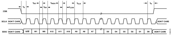
Figure 74. Serial Port Interface Timing Diagram
