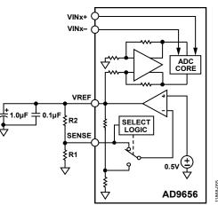
Figure 52. Programmable Internal Reference Configuration
