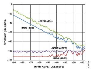
Figure 29. Two-Tone SFDR/IMD3 vs. Input Amplitude (A\_IN) with  $f_{\rm IN1}=70.5$  MHz and  $f_{\rm IN2}=72.5$  MHz,  $f_{\rm SAMPLE}=125$  MSPS,  $V_{\rm REF}=1.0$  V
