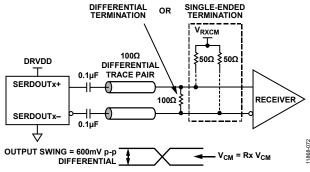
Figure 71. AC-Coupled Digital Output Termination Example
