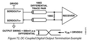
If there is no far-end receiver termination, or if there is poor differential trace routing, timing errors can result. To avoid such timing errors, it is recommended that the trace length be less than six inches and the differential output traces be close together and of equal lengths.
