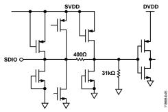
Figure 39. Equivalent SDIO Input Circuit
