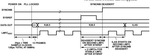
Figure 65. JESD204B Tx Start-Up and Synchronization Timing
