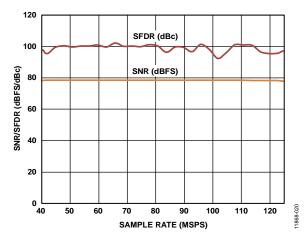
Figure 35. SNR/SFDR vs. Sample Rate,  $f_{IN} = 9.7 \text{ MHz}$ ,  $V_{REF} = 1.0 \text{ V}$
