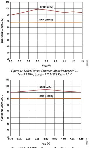
Figure 48. SNR/SFDR vs. Common-Mode Voltage (V<sub>CM</sub>), f<sub>IN</sub> = 9.7 MHz, f<sub>SAMPLE</sub> = 125 MSPS, V<sub>REF</sub> = 1.4 V
