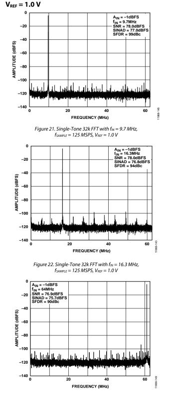
Figure 23. Single-Tone 32k FFT with  $f_{IN} = 64$  MHz,  $f_{SAMPLE} = 125$  MSPS,  $V_{REF} = 1.0$  V
