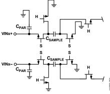
Figure 46. Switched-Capacitor Input Circuit
