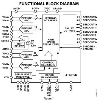
The AD9656 is available in an RoHS compliant, nonmagnetic, 56-lead LFCSP. It is specified over the  $-40^{\circ}$ C to  $+85^{\circ}$ C industrial temperature range.
