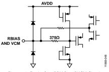
Figure 43. Equivalent RBIAS and VCM Circuit
