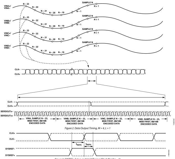
Figure 3. SYSREF± Setup and Hold Timing (Clock Divider = 1)
