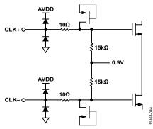
Figure 38. Equivalent Clock Input Circuit
