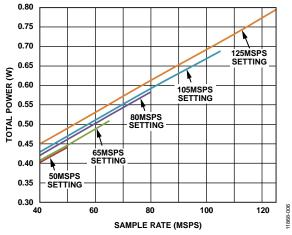
Figure 63. Total Power vs.  $f_{SAMPLE}$  for  $f_{IN} = 9.7$  MHz, Four Channels ( $V_{REF} = 1.4$  V)
