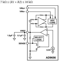
Figure 51. 1.0 V Internal Reference Configuration
