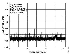
Figure 26. Single-Tone 32k FFT with  $f_{IN}$  = 301 MHz,  $f_{SAMPLE}$  = 125 MSPS,  $V_{REF}$  = 1.0 V
