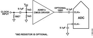
Figure 61. Single-Ended 1.8 V CMOS Input Clock (Up to 200 MHz)
