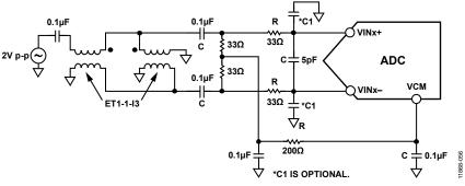
Figure 49. Differential Double Balun Input Configuration for Baseband Applications
