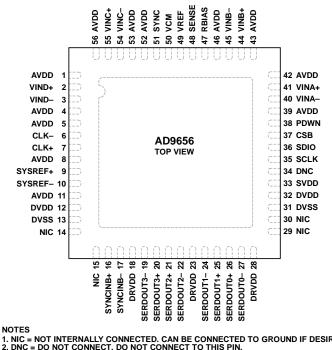
1. NIC = NOT INTERNALLY CONNECTED. CAN BE CONNECTED TO GROUND IF DESIRED. 2. DNC = DO NOT CONNECT. DO NOT CONNECT TO THIS PIN. 3. THE EXPOSED THERMAL PAD ON THE BOTTOM OF THE PACKAGE PROVIDES THE ANALOG GROUND FOR THE PART. THIS EXPOSED PAD MUST BE CONNECTED TO GROUND FOR PROPER OPERATION.
