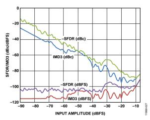
Figure 13. Two-Tone SFDR/IMD3 vs. Input Amplitude (A<sub>IN</sub>) with  $f_{IN1} = 70.5$  MHz and  $f_{IN2} = 72.5$  MHz,  $f_{SAMPLE} = 125$  MSPS,  $V_{REF} = 1.4$  V
