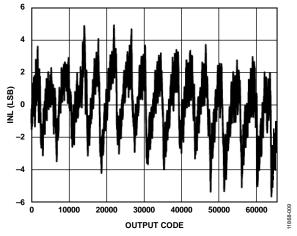
Figure 32. Integral Nonlinearity (INL),  $f_{IN} = 9.7 \text{ MHz}$ ,  $f_{SAMPLE} = 125 \text{ MSPS}$ ,  $V_{REF} = 1.0 \text{ V}$
