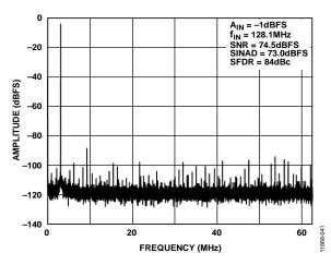
Figure 24. Single-Tone 32k FFT with  $f_{IN} = 128.1$  MHz,  $f_{SAMPLE} = 125$  MSPS,  $V_{REF} = 1.0$  V
