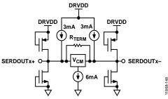
Figure 40. Equivalent SERDOUTx± Circuit
