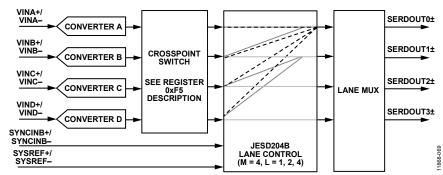
Figure 68. AD9656 Transmit Link Simplified Conceptual Block Diagram
