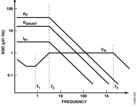
Figure 127. Photodiode TIA RTO Noise Spectral Density
