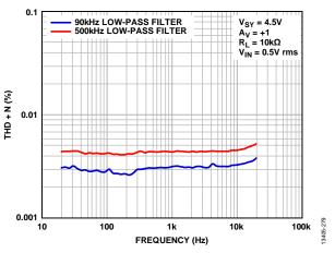
Figure 79. THD + N vs. Frequency,  $V_{SY} = 4.5 V$
