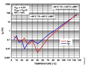
Figure 34. Input Bias Current (I<sub>B</sub>) vs. Temperature,  $V_{SY} = 4.5 V$
