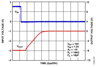
Figure 72. Negative Overload Recovery,  $V_{SY} = 16 V$
