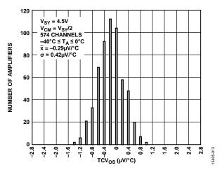
Figure 10. Input Offset Voltage Drift Distribution,  $-40^{\circ}C \le T_A \le 0^{\circ}C$ ,  $V_{SY} = 4.5 V$
