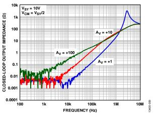
Figure 59. Closed-Loop Output Impedance vs. Frequency
