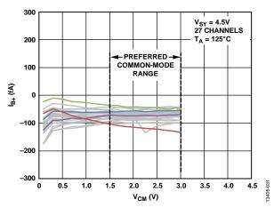
Figure 31. Noninverting Input Bias Current ( $I_{B+}$ ) vs. Common-Mode Voltage ( $V_{CM}$ ),  $V_{SY} = 4.5 V$ ,  $T_A = 125^{\circ}C$
