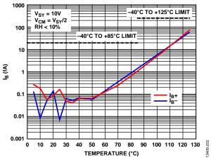
Figure 2. Input Bias Current ( $I_B$ ) vs. Temperature,  $V_{SY} = 10 V$
