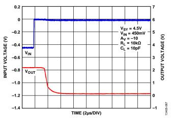
Figure 67. Positive Overload Recovery,  $V_{SY} = 4.5 V$
