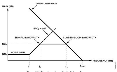
Figure 126. Transimpedance Noise Gain vs. Frequency
