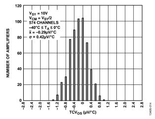
Figure 11. Input Offset Voltage Drift Distribution,  $-40^{\circ}C \le T_A \le 0^{\circ}C$ ,  $V_{SY} = 10 V$
