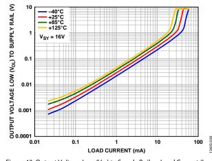
Figure 42. Output Voltage Low ( $V_{OL}$ ) to Supply Rail vs. Load Current ( $I_{LOAD}$ ),  $V_{SY} = 16 V$
