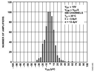
Figure 88. Input Offset Voltage Distribution, V<sub>SY</sub> = 10 V
