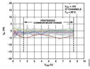
Figure 23. Inverting Input Bias Current (I<sub>B-</sub>) vs. Common-Mode Voltage ( $V_{CM}$ ),  $V_{SY} = 10 V$ ,  $T_A = 85^{\circ}C$
