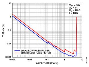
Figure 84. THD + N vs. Amplitude,  $V_{SY} = 16 V$
