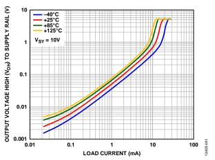
Figure 44. Output Voltage High (V<sub>OH</sub>) to Supply Rail vs. Load Current (I<sub>LOAD</sub>),  $V_{SY} = 10 V$
