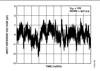
Figure 86. 0.1 Hz to 10 Hz Noise
