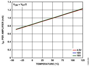
Figure 53. Supply Current (I<sub>sy</sub>) per Amplifier vs. Temperature
