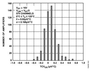
Figure 98. Input Offset Voltage Drift Distribution,  $0^{\circ}C \le T_A \le 125^{\circ}C$ ,  $V_{SY} = 16 V$
