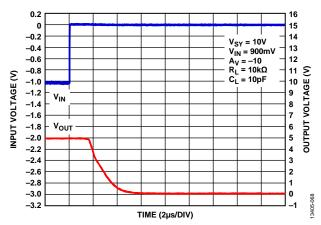
Figure 68. Positive Overload Recovery,  $V_{SY} = 10 V$
