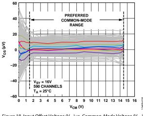
Figure 18. Input Offset Voltage (V\_{CS}) vs. Common-Mode Voltage (V\_{CM}),  $V_{SY} = 16 V$
