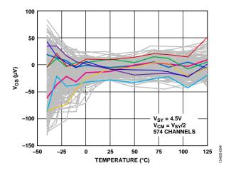
Figure 90. Input Offset Voltage ( $V_{OS}$ ) vs. Temperature,  $V_{SY} = 4.5 V$
