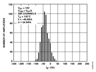
Figure 37. Inverting Input Bias Current Histogram,  $T_A = 125$  °C,  $V_{SY} = 10$  V
