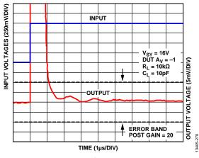
Figure 78. Positive Settling Time to 0.1%,  $V_{SY} = 16 V$
