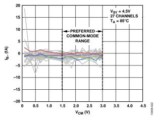
Figure 22. Inverting Input Bias Current ( $I_{B-}$ ) vs. Common-Mode Voltage ( $V_{CM}$ ),  $V_{SY} = 4.5 V$ ,  $T_A = 85^{\circ}C$
