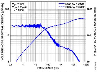
Figure 132. RTO Noise Spectral Density (60°C)
