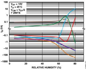
Figure 112. Effective Input Bias Current vs. Relative Humidity
