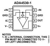
Figure 3. Pin Configuration
