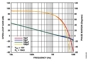
Figure 55. Open-Loop Gain and Phase Margin vs. Frequency
