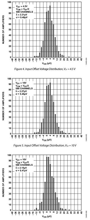
Figure 6. Input Offset Voltage Distribution,  $V_{SY} = 16 V$
