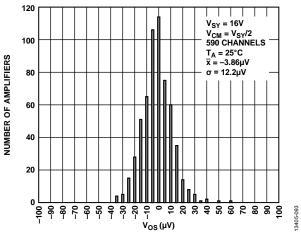
Figure 89. Input Offset Voltage Distribution, V<sub>SY</sub> = 16 V
