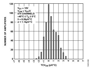
Figure 94. Input Offset Voltage Drift Distribution,  $-40^{\circ}C \le T_A \le 0^{\circ}C$ ,  $V_{SY} = 10 V$
