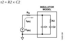
Figure 108. Dielectric Relaxation Model Test Circuit
