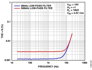
Figure 81. THD + N vs. Frequency,  $V_{SY} = 16 V$
