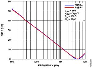
Figure 57. PSRR vs. Frequency
