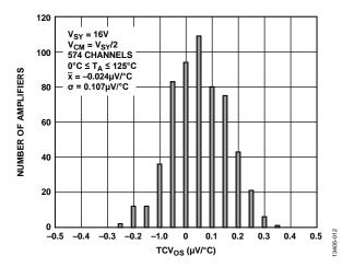
Figure 15. Input Offset Voltage Drift Distribution,  $0^{\circ}C \le T_A \le 125^{\circ}C$ ,  $V_{SY} = 16 V$
