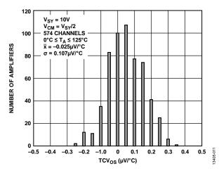
Figure 14. Input Offset Voltage Drift Distribution,  $0^{\circ}C \le T_A \le 125^{\circ}C$ ,  $V_{SY} = 10 V$
