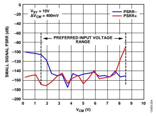
Figure 54. Small Signal PSRR vs. Common-Mode Voltage ( $V_{CM}$ )
