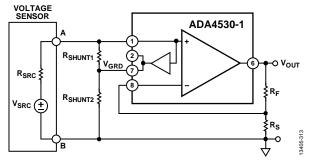
Figure 107. Voltage Buffer Circuit with Guard
