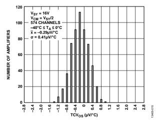
Figure 12. Input Offset Voltage Drift Distribution,  $-40^{\circ}C \le T_A \le 0^{\circ}C$ ,  $V_{SY} = 16 V$
