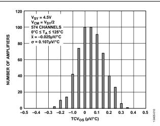
Figure 13. Input Offset Voltage Drift Distribution,  $0^{\circ}C \le T_A \le 125^{\circ}C$ ,  $V_{SY} = 4.5 V$
