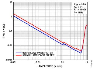
Figure 82. THD + N vs. Amplitude,  $V_{SY} = 4.5 V$
