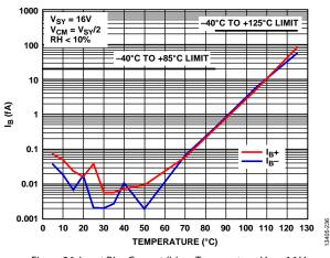
Figure 36. Input Bias Current (I<sub>B</sub>) vs. Temperature,  $V_{SY} = 16 V$
