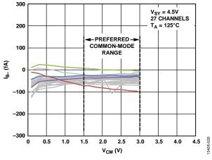
Figure 28. Inverting Input Bias Current (I\_B-) vs. Common-Mode Voltage (V\_CM),  $V_{SY}$  = 4.5 V,  $T_A$  = 125 °C
