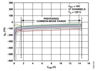
Figure 33. Noninverting Input Bias Current ( $I_{B+}$ ) vs. Common-Mode Voltage ( $V_{CM}$ ),  $V_{SY} = 16$  V,  $T_A = 125$  °C
