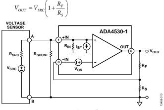
Figure 105. Voltage Buffer Circuit
