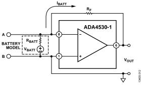
Figure 115. TIA Circuit with Contamination Battery
