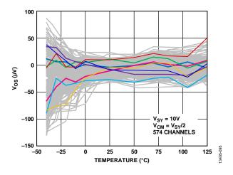
Figure 91. Input Offset Voltage ( $V_{OS}$ ) vs. Temperature,  $V_{SY} = 10 V$
