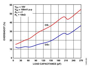
Figure 60. Small Signal Overshoot vs. Load Capacitance
