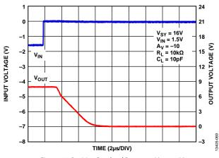
Figure 69. Positive Overload Recovery,  $V_{SY} = 16 V$
