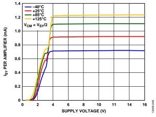
Figure 52. Supply Current (Isy) per Amplifier vs. Supply Voltage (Vsy)
