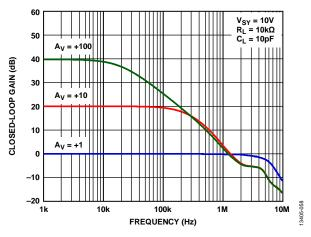
Figure 58. Closed-Loop Gain vs. Frequency
