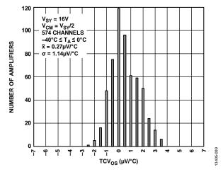
Figure 95. Input Offset Voltage Drift Distribution,  $-40^{\circ}C \le T_A \le 0^{\circ}C$ ,  $V_{SY} = 16 V$
