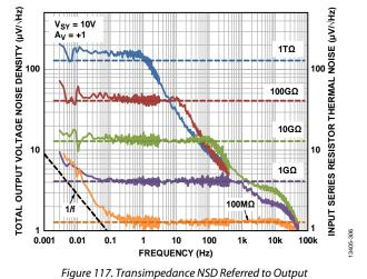
$V_{\text{NRTO}}$  is dominated by the resistor noise for all of the test resistors up 1 T $\Omega$ . This means that the current noise contribution from the ADA4530-1 is insignificant relative to the thermal noise of these resistors.
