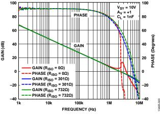
Figure 103. Frequency Response with C<sub>L</sub> = 1 nF and Various Isolating Resistors
