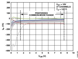
Figure 29. Inverting Input Bias Current (I<sub>B</sub>.) vs. Common-Mode Voltage ( $V_{CM}$ ),  $V_{SY} = 10 V$ ,  $T_A = 125 ^{\circ}$ C
