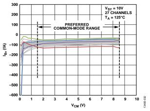
Figure 32. Noninverting Input Bias Current ( $I_{B+1}$ ) vs. Common-Mode Voltage ( $V_{CM}$ ),  $V_{SY} = 10 V$ ,  $T_A = 125 ^{\circ}$ C
