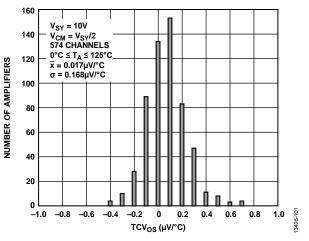
Figure 97. Input Offset Voltage Drift Distribution,  $0^{\circ}C \le T_A \le 125^{\circ}C$ ,  $V_{SY} = 10 V$
