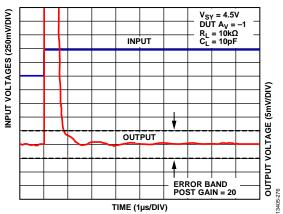
Figure 76. Positive Settling Time to 0.1%,  $V_{SY} = 4.5 V$
