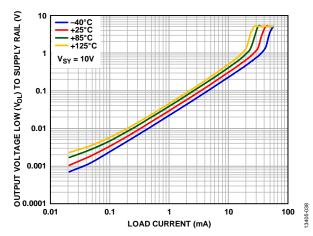
Figure 41 Output Voltage Low (V<sub>OL</sub>) to Supply Rail vs. Load Current ( $I_{LOAD}$ ),  $V_{SY} = 10 V$
