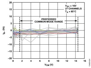
Figure 24. Inverting Input Bias Current (I<sub>B-</sub>) vs. Common-Mode Voltage (V<sub>CM</sub>),  $V_{SY} = 16 V, T_A = 85 ^{\circ}C$
