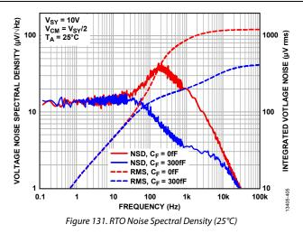
The dashed curves show the integration of the NSD across the frequency spectrum. These are useful to calculate the rms noise over a variety of bandwidths. For example, the rms noise over the entire 100 kHz measurement bandwidth is 400  $\mu$ V rms, which is approximately the same as the calculated total noise of 333  $\mu$ V rms. If a postfilter is added with a noise bandwidth of 1 kHz, Figure 131 shows that the integrated noise is 200  $\mu$ V rms (a 2× improvement).
