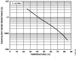
Figure 120. Equivalent Noise Resistance vs. Temperature
