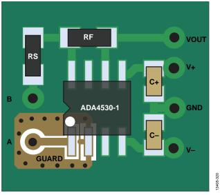
Figure 121. Buffer Circuit Layout
