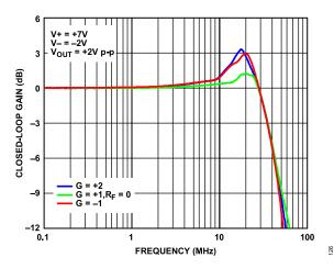
Figure 24. ADC Driver Large Signal Frequency Response for Various Gains
