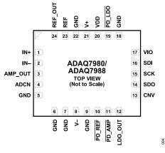
Figure 4. Pin Configuration
