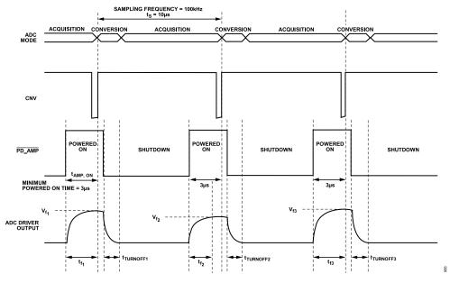
Figure 63. Timing Waveforms
