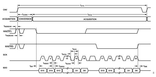
Figure 76. 4-Wire CS Mode Without the Busy Indicator Serial Interface Timing
