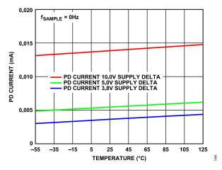
Figure 41. Total ADC Driver and Reference Buffer Power-Down (PD) Current vs. Temperature
