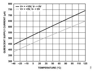
Figure 28. ADC Driver and Reference Buffer Quiescent Supply Current vs. Temperature for Various Supplies
