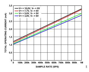
Figure 44. Total Operating Current vs. Sample Rate for Various Supplies
