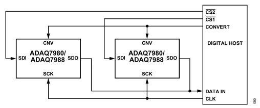
Figure 75. 4-Wire CS Mode Without the Busy Indicator Connection Diagram
