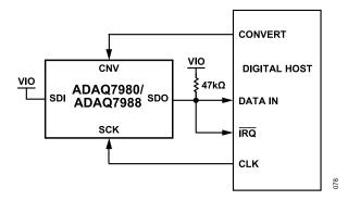
Figure 73. 3-Wire CS Mode with the Busy Indicator Connection Diagram (SDI = 1, High)
