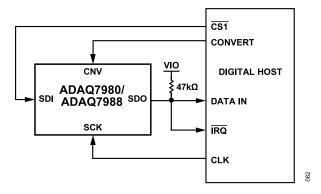
Figure 77. 4-Wire CS Mode with the Busy Indicator Connection Diagram
