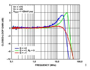
Figure 20. ADC Driver Small Signal Frequency Response for Various Gains
