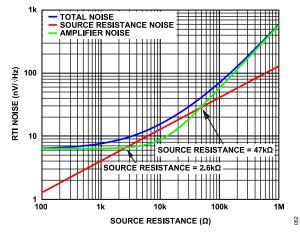
Figure 59. RTI Noise vs. Source Resistance
