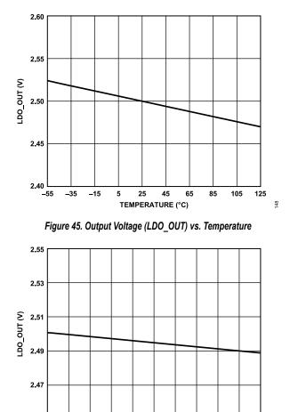
LOAD CURRENT (mA) Figure 46. Output Voltage (LDO\_OUT) vs. Load Current (I<sub>LOAD</sub>)
