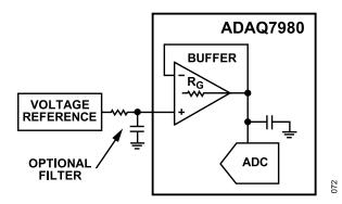
Figure 67. Voltage Reference with RC Filtering
