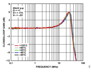
Figure 23. ADC Driver Small Signal Frequency Response for Various Temperatures
