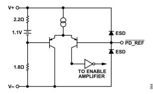
Figure 68. Reference Buffer Shutdown Circuit
