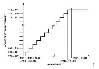
Figure 53. ADC Ideal Transfer Function
