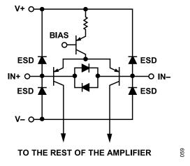
Figure 56. ADC Driver Input Stage and Protection Diodes
