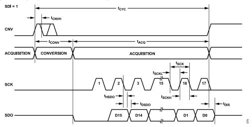
Figure 74. 3-Wire CS Mode with the Busy Indicator Serial Interface Timing (SDI = 1, High)
