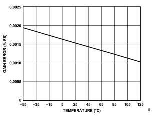
Figure 37. Gain Error vs. Temperature
