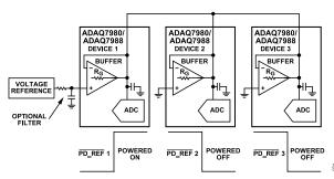
Figure 69. Reference Configuration for Multiple ADAQ7980/ADAQ7988 Devices
