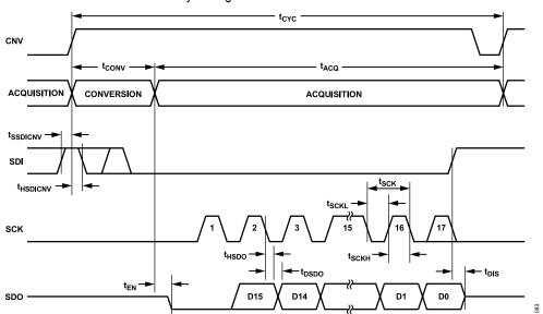
Figure 78. 4-Wire CS Mode with the Busy Indicator Serial Interface Timing
