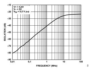
Figure 51. Forward/Off Isolation vs. Frequency
