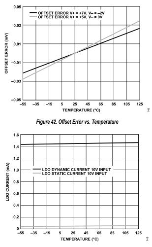
Figure 43. LDO Current vs. Temperature for Various Supplies
