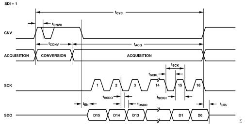
Figure 72. 3-Wire CS Mode Without the Busy Indicator Serial Interface Timing (SDI = 1, High)
