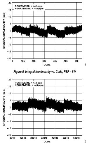
Figure 6. Integral Nonlinearity vs. Code, V+ = VDD = 5 V, V- = 0 V, REF = 3.3 V
