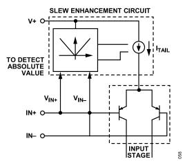
Figure 55. ADC Driver Slew Enhancement Circuit
