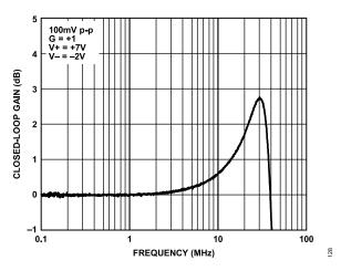
Figure 26. ADC Driver Small Signal 0.1 dB Bandwidth
