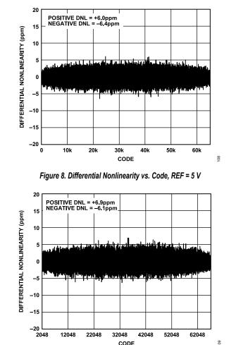
Figure 9. Differential Nonlinearity vs. Code, V+ = VDD = 5 V, V- = 0 V, REF = 3.3 V
