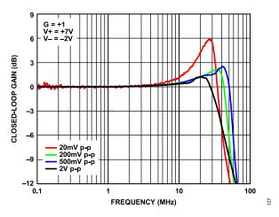
Figure 25. Frequency Response for Various Output Voltages
