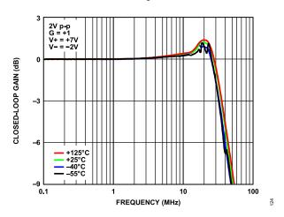
Figure 22. Large Signal Frequency Response for Various Temperatures
