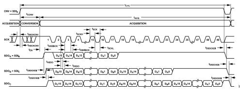
Figure 82. Chain Mode with Busy Indicator Serial Interface Timing
