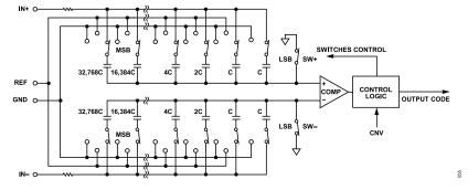
Figure 52. ADC Simplified Schematic
