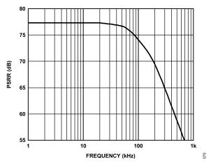
Figure 70. PSRR vs. Frequency
