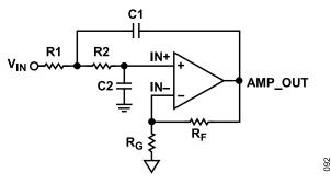
Figure 87. Schematic of a Second-Order, Low-Pass Active Filter
