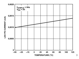
Figure 48. LDO PD Current vs. Temperature
