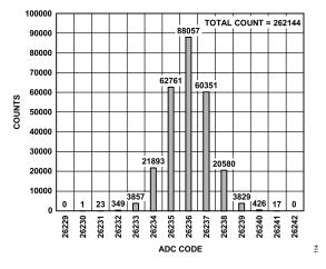
Figure 14. Histogram of a DC Input at the Code Center, REF = 2.5 V
