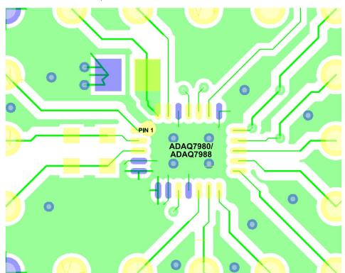
Figure 89. Example Layout for the ADAQ7980/ADAQ7988
