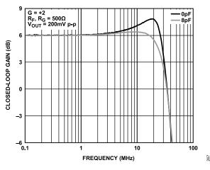
Figure 66. Peaking Mitigation in Small Signal Frequency Response
