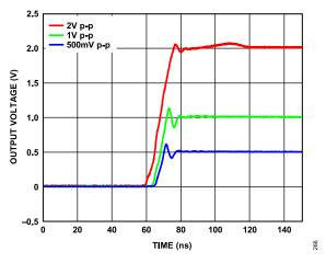
Figure 65. Step Response with Selected Output Steps
