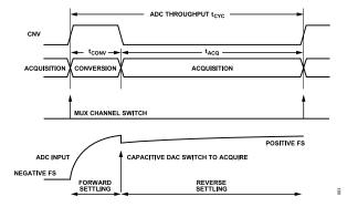
Figure 60. Multiplexed Application Timing
