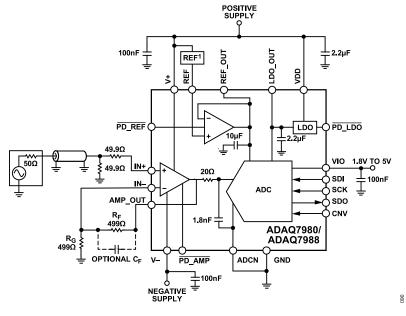
Figure 85. Noninverting ADC Driver, Gain = 2
