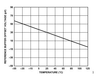
Figure 38. Reference Buffer Input Offset Voltage vs. Temperature
