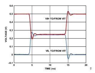
Figure 16. Driver Active (VIH/VIL) to/from VTERM Transition; VIH = 1.0 V, VIT = 0.5 V; VIL = 0.0 V,  $50 \Omega$  Termination
