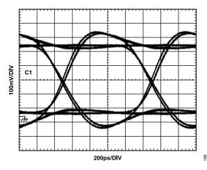
Figure 97. Driver Eye Diagram, 2000 Mbps, PRBS31; VIH = 1 V, VIL = 0 V
