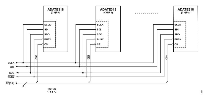
Figure 113. Multiple SPI with Shared SDO Line
