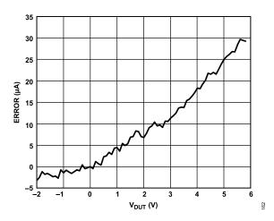
Figure 69. PPMU Force Current Range A Compliance Error at +40 mA vs.
