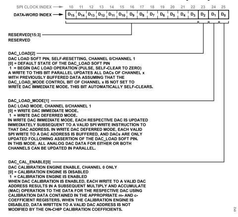
Figure 116. DAC Control Register (ADDR = 0x11)
