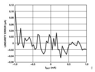
Figure 79. PPMU Range B Measure Current Linearity Error
