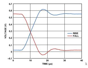
Figure 112. PPMU Transient Response, FV Range C, 0 V to 0.5 V, Uncalibrated,  $C_{\rm LOAD}$  = 2000 pF
