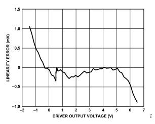
Figure 26. Driver VIT Linearity Error
