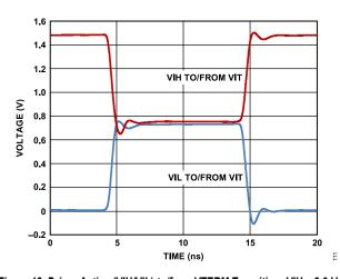
Figure 18. Driver Active (VIH/VIL) to/from VTERM Transition; VIH = 3.0 V, VIT = 1.5 V; VIL = 0.0 V,  $50 \Omega$  Termination
