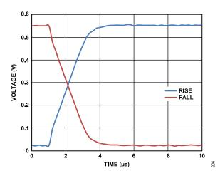
Figure 111. PPMU Transient Response, FV Range A, 0 V to 0.5 V, Uncalibrated,  $C_{LOAD}$  = 2000 pF
