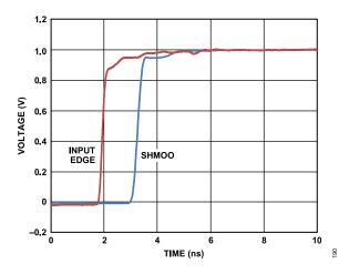
Figure 42. Normal Window Comparator Shmoo; 1.0 V Swing, 50 Ω Termination, 200 ps (20% to 80%)
