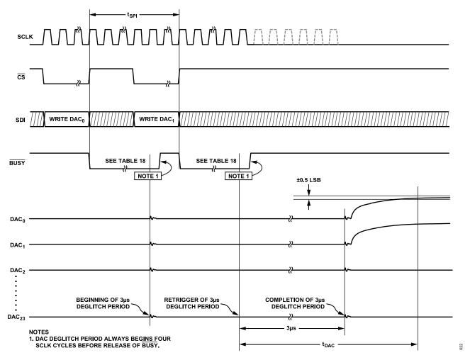
Figure 126. SPI DAC Write and Settling Time
