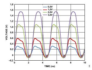
Figure 14. 400 MHz Driver Response, VIH = 0.5 V, 1.0 V, 2.0 V, 3.0 V; VIL = 0.0 V, 50  $\Omega$  Termination
