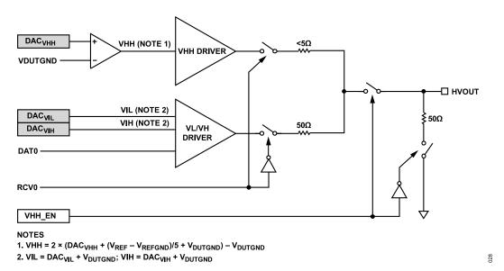
Figure 131. VHH and VIL/VIH Driver Block Diagram
