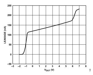
Figure 56. DUTx Pin Leakage in High-Z Mode
