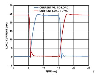
Figure 50. Active Load Response to/from Drive VIL = 0 V, 50  $\Omega$  Termination, IOL = 25 mA, VCOM = 2 V
