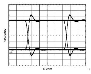
Figure 92. Driver Eye Diagram, 400 Mbps, PRBS31; VIH = 1 V, VIL = 0 V
