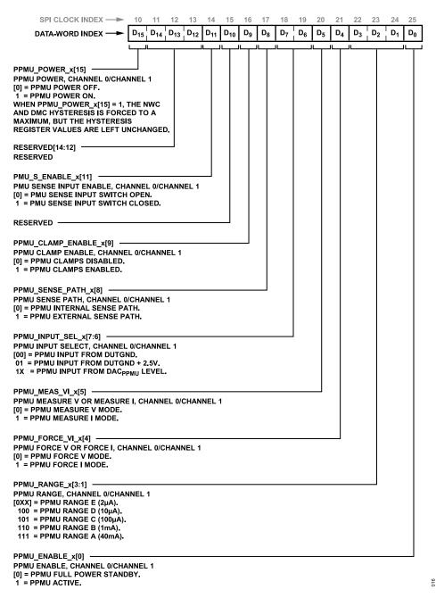
Figure 120. PPMU Control Register (ADDR = 0x1A)
