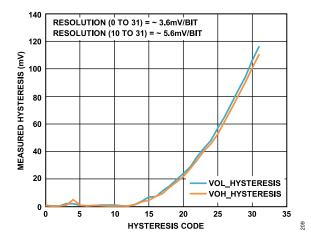
Figure 91. Differential Comparator Hysteresis Transfer Function
