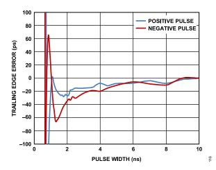
Figure 23. Driver Trailing Edge Timing Error vs. Pulse Width, VIH = 3.0 V; VIL = 0.0 V, 50  $\Omega$  Termination
