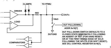
Figure 114. DUTx to VDUTGND Soft Connect Detail
