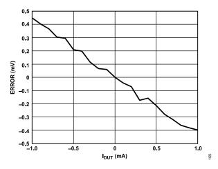
Figure 66. PPMU Force Voltage Range B Compliance Error at -2.0 V vs.
