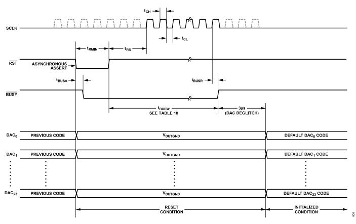
Figure 4. SPI Detailed Hardware Reset Timing Diagram
