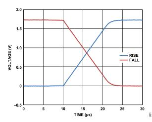
Figure 106. PPMU Transient Response, FI Range B, Full-Scale Transition, Uncalibrated,  $C_{LOAD}$  = 200 pF,  $R_{LOAD}$  = 1.5 k $\Omega$
