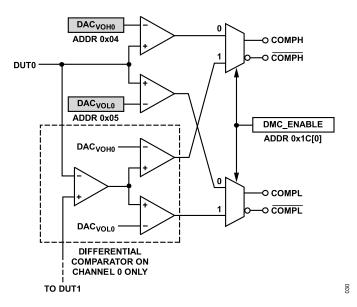
Figure 133. Comparator Block Diagram
