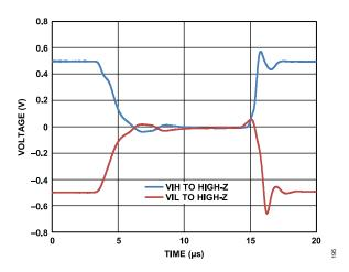
Figure 99. Drive to/from High-Z Transition, VIH = 1 V, VIL = -1 V, 50  $\Omega$ Termination
