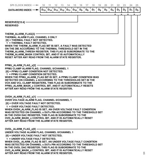
Figure 124. Alarm State Register (ADDR = 0x1E) (Read Only)
