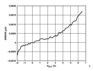
Figure 72. PPMU Force Current Range E Compliance Error at -2 μA vs.
