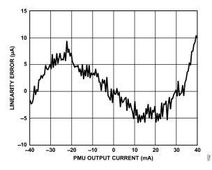
Figure 59. PPMU Range A Force Current Linearity Error
