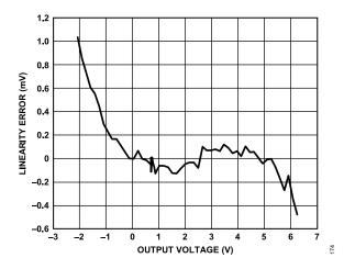
Figure 81. Reflection Clamp VCL Linearity Error
