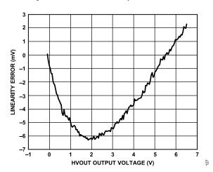
Figure 34. HVOUT VIH Linearity Error
