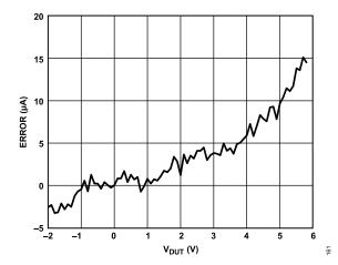
Figure 68. PPMU Force Current Range A Compliance Error at -40 mA vs.
