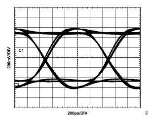
Figure 98. Driver Eye Diagram, 2000 Mbps, PRBS31; VIH = 2 V, VIL = 0 V
