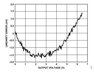
Figure 84. PPMU Voltage Clamp VCH Linearity Error
