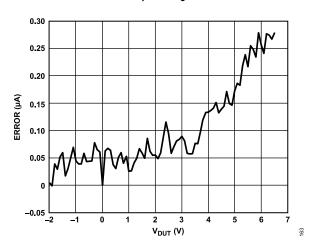
Figure 70. PPMU Force Current Range B Compliance Error at −1 mA vs.
