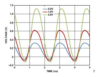
Figure 15. 600 MHz Driver Response, VIH = 0.5 V, 1.0 V, 2.0 V; VIL = 0.0 V, 50  $\Omega$  Termination
