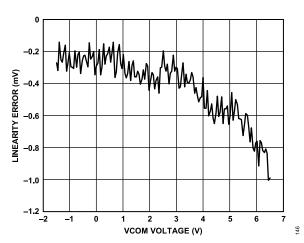
Figure 53. Active Load VCOM Linearity Error
