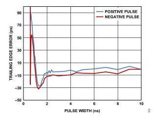
Figure 20. Driver Trailing Edge Timing Error vs. Pulse Width, VIH = 0.5 V; VIL = 0.0 V, 50  $\Omega$  Termination
