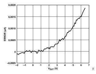
Figure 73. PPMU Force Current Range E Compliance Error at +2 μA vs.
