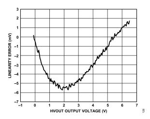
Figure 35. HVOUT VIL Linearity Error
