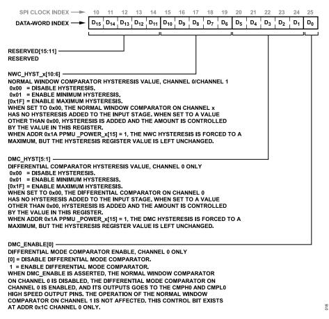
Figure 122. CMP Control Register (ADDR = 0x1C)
