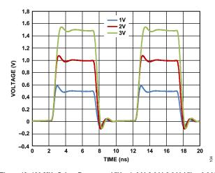
Figure 12. 100 MHz Driver Response, VIH = 1. 0 V, 2.0 V, 3.0 V; VIL = 0.0 V, 50  $\Omega$  Termination
