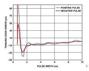
Figure 19. Driver Trailing Edge Timing Error Pulse Width, VIH = 0.2 V; VIL = 0.0 V,  $50 \Omega$  Termination
