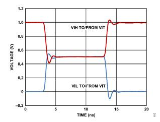
Figure 17. Driver Active (VIH/VIL) to/from VTERM Transition; VIH = 2.0 V, VIT = 1.0 V; VIL = 0.0 V,  $50 \Omega$  Termination
