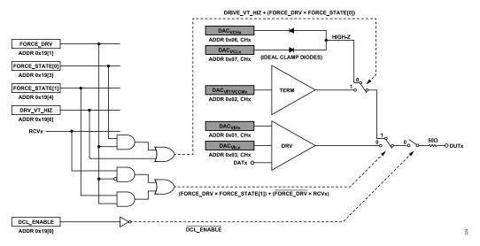
Figure 127. Driver Block Diagram
