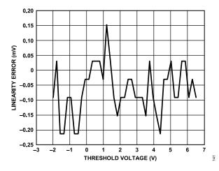
Figure 48. PPMU Go/No-Go Comparator Linearity Error
