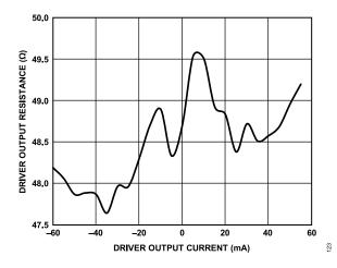
Figure 30. Driver Output Resistance vs. Output Current
