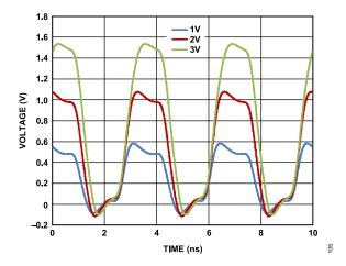
Figure 13. 300 MHz Driver Response, VIH = 1.0 V, 2.0 V, 3.0 V; VIL = 0.0 V, 50  $\Omega$  Termination
