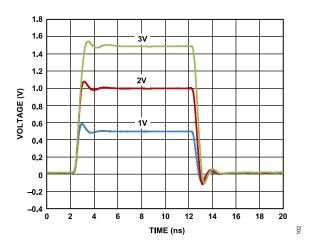
Figure 10. Driver Large Signal Response, VIH = 1.0 V, 2.0 V, 3.0 V; VIL = 0.0 V, 50  $\Omega$  Termination
