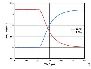
Figure 107. PPMU Transient Response, FI Range C, Full-Scale Transition, Uncalibrated,  $C_{LOAD}$  = 200 pF,  $R_{LOAD}$  = 15 k $\Omega$
