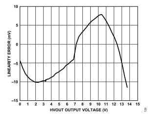
Figure 36. HVOUT VHH Linearity Error
