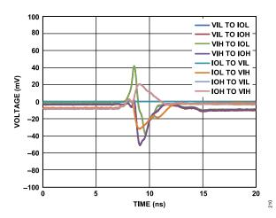
Figure 100. Drive to/from Active Load Transient, VIL = VIH = 0 V, IOH = IOL = 0 V
