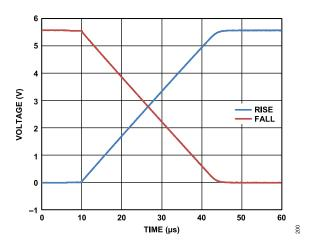
Figure 105. PPMU Transient Response, FI Range A, Full -Scale Transition, Uncalibrated,  $C_{LOAD}$  = 200 pF,  $R_{LOAD}$  = 120  $\Omega$
