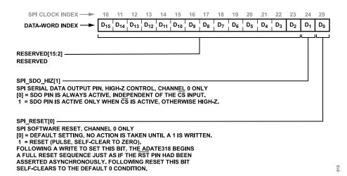
Figure 117. SPI Control Register (ADDR = 0x12)
