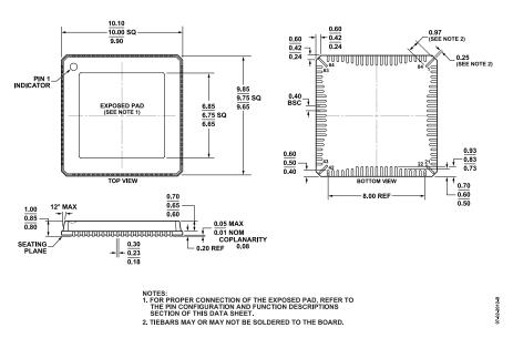
Figure 137. 84-Lead Lead Frame Chip Scale Package [LFCSP] 10 mm × 10 mm Body and 0.85 mm Package Height (CP-84-2) Dimensions shown in millimeters
