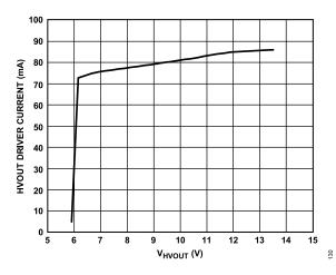
Figure 37. HVOUT VHH Output Current Limit; VHH = 5.9 V, HVOUT Swept 5.9 V to 13.5 V
