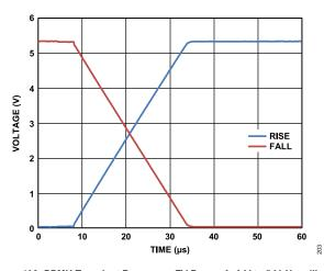
Figure 108. PPMU Transient Response, FV Range A, 0 V to 5 V, Uncalibrated,  $C_{LOAD} = 200 \text{ pF}$
