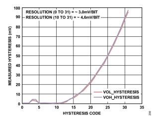
Figure 90. Normal Window Comparator Hysteresis Transfer Function
