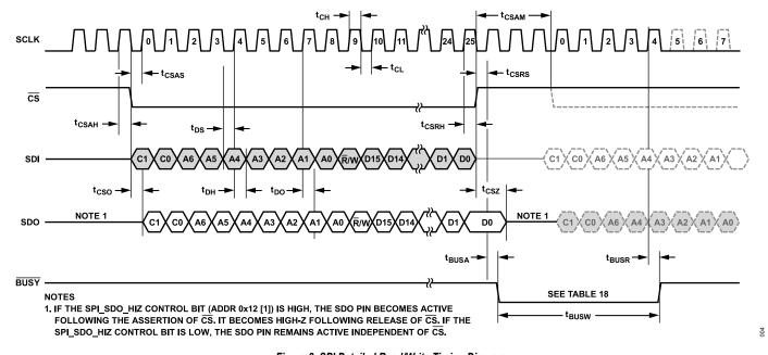
Figure 2. SPI Detailed Read/Write Timing Diagram
