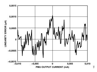
Figure 62. PPMU Range D Force Current Linearity Error
