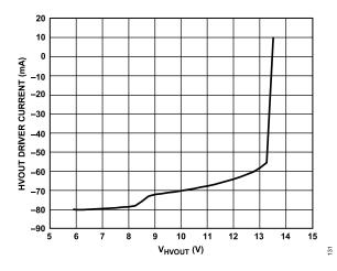
Figure 38. HVOUT VHH Output Current Limit; VHH = 13.5 V, HVOUT Swept 5.9 V to 13.5 V
