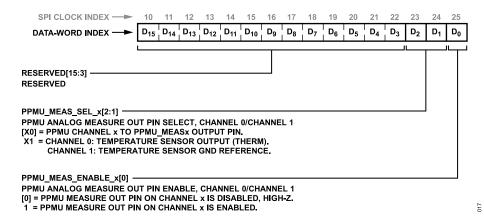
Figure 121. PPMU MEAS Control Register (ADDR = 0x1B)
