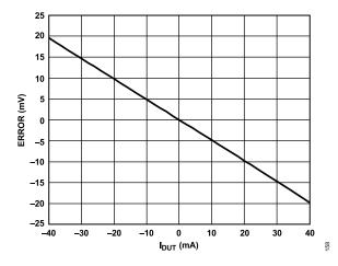
Figure 65. PPMU Force Voltage Range A Compliance Error at +5.75 V vs.
