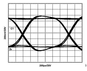
Figure 96. Driver Eye Diagram, 1600 Mbps, PRBS31; VIH = 2 V, VIL = 0 V
