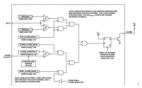
Figure 136. Fault Alarm Block Diagram
