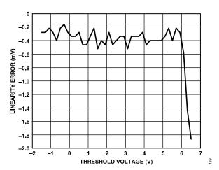
Figure 46. Normal Window Comparator Threshold Linearity Error
