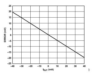
Figure 64. PPMU Force Voltage Range A Compliance Error at −2.0 V vs.
