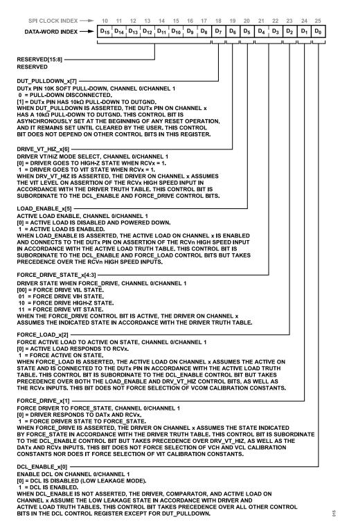
Figure 119. DCL Control Register (ADDR = 0x19)
