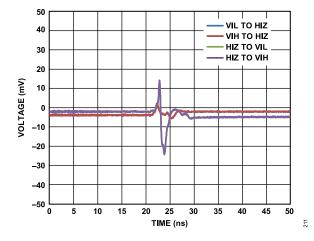
Figure 101. Drive to/from High-Z Transient, VIL = VIH = 0 V, 50  $\Omega$  Termination
