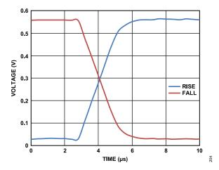
Figure 109. PPMU Transient Response, FV Range A, 0 V to 0.5 V, Uncalibrated, C<sub>LOAD</sub> = 200 pF
