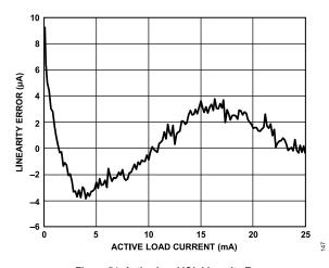
Figure 54. Active Load IOL Linearity Error
