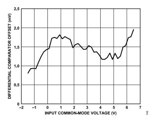
Figure 49. Differential Comparator CMR Error
