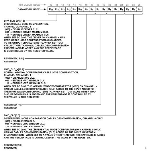
Figure 125. CLC Control Register (ADDR = 0x1F)
