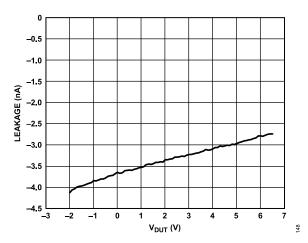
Figure 55. DUTx Pin Leakage in Low Leakage Mode
