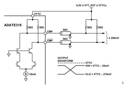
Figure 134. Comparator Output Stage Diagram
