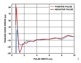
Figure 22. Driver Trailing Edge Timing Error vs. Pulse Width, VIH = 2.0 V; VIL = 0.0 V, 50  $\Omega$  Termination
