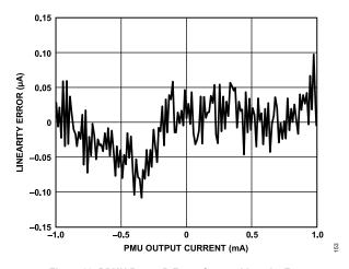
Figure 60. PPMU Range B Force Current Linearity Error
