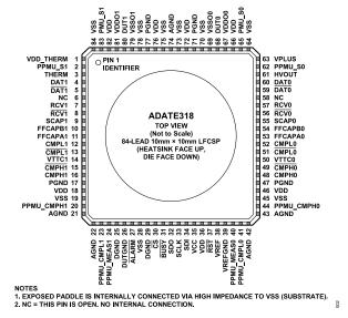
Figure 8. LFCSP Pin Configuration
