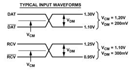
Figure 128. Driver Input Stage Diagram
