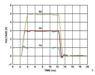
Figure 11. Driver Large Signal Response, VIH = 1.0 V, 3.0 V, 5.0 V; VIL = 0.0 V,  $50 \Omega$  Unterminated
