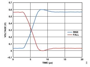
Figure 110. PPMU Transient Response, FV Range C, 0 V to 0.5 V, Uncalibrated,  $C_{LOAD}$  = 200 pF
