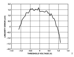
Figure 47. Differential Comparator Threshold Linearity Error
