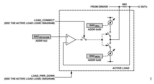
Figure 129. Active Load Block Diagram
