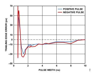
Figure 21. Driver Trailing Edge Timing Error vs. Pulse Width, VIH = 1.0 V; VIL = 0.0 V, 50  $\Omega$  Termination
