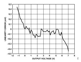
Figure 82. Reflection Clamp VCH Linearity Error
