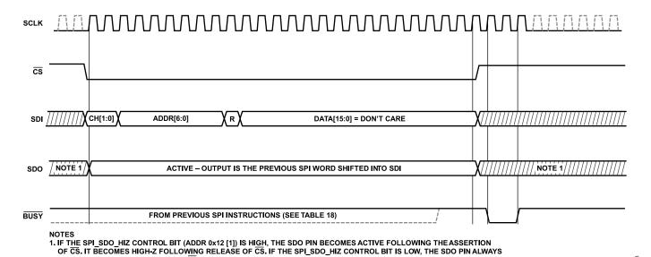
Figure 6. SPI Read Request Instruction (Prior to Readout)
