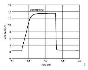
Figure 33. HVOUT Transient Response, VHH = 13.5 V
