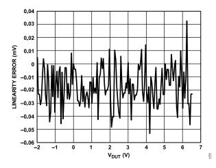
Figure 78. PPMU Range B Measure Voltage Linearity Error
