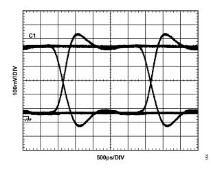
Figure 93. Driver Eye Diagram, 800 Mbps, PRBS31; VIH = 1 V, VIL = 0 V
