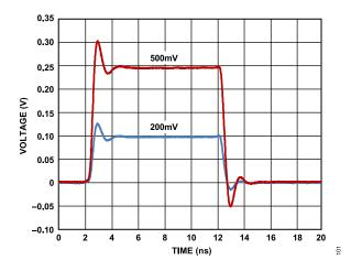
Figure 9. Driver Small Signal Response, VIH = 0.2 V, 0.5 V; VIL = 0.0 V, 50  $\Omega$  Termination
