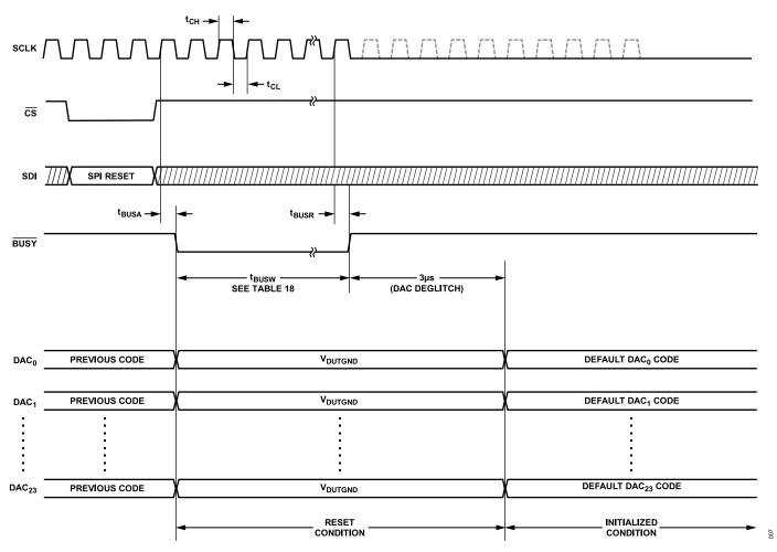
Figure 5. SPI Detailed Software Reset Timing Diagram
