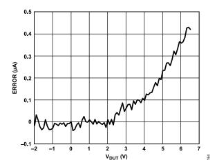
Figure 71. PPMU Force Current Range B Compliance Error at +1 mA vs.
