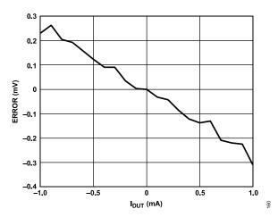
Figure 67. PPMU Force Voltage Range B Compliance Error at +6.5 V vs.
