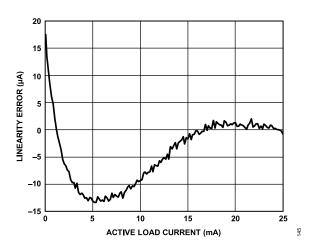
Figure 52. Active Load IOH Linearity Error
