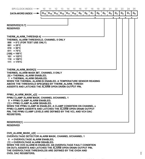
Figure 123. Alarm Mask Register (ADDR = 0x1D)
