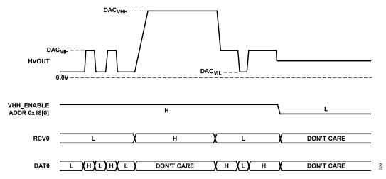
Figure 132. VHH and VIL/VIH Waveform Diagram
