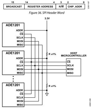
Figure 37. Multichip SPI Addressing Mode
