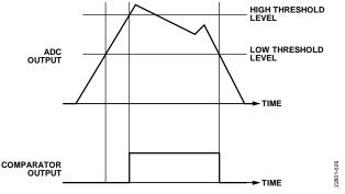
Figure 25. Comparator Behavior in Hysteretic Output Mode
