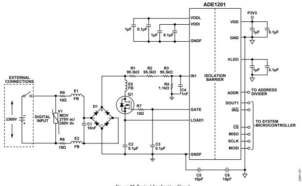
Figure 20. Typical Application Circuit
