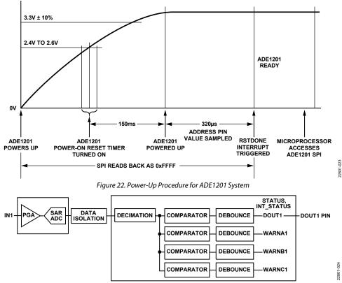
Figure 23. Digital Input Signal Path
