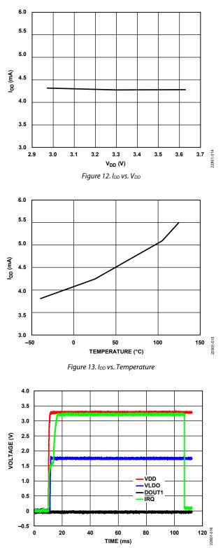
Figure 14. Power-Up of Nonisolated Side (VDD, VLDO, DOUT1, and IRQ Pins)
