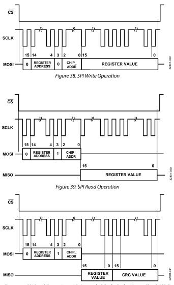
Figure 40. SPI Read Operation with Appended Cyclic Redundancy Check (CRC)
