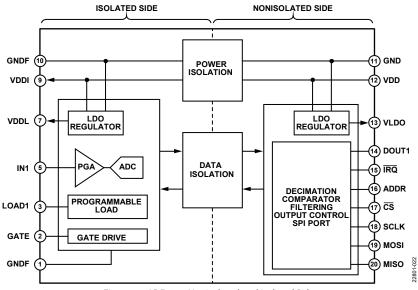
Figure 21. ADE1201 Nonisolated and Isolated Sides
