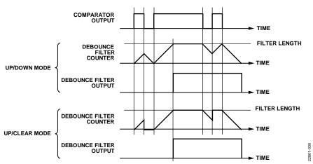
Figure 29. Debounce Filter Function Example
