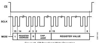
Figure 41. SPI Broadcast Write Operation
