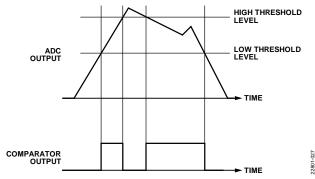
Figure 26. Comparator Behavior in Midrange Output Mode
