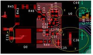
Figure 46. Close Up of the ADE1201 Support Circuitry
