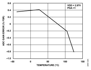
Figure 19. ADC Gain Error vs. Temperature
