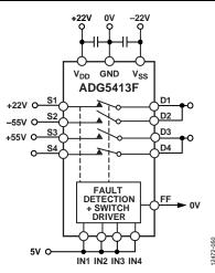
Figure 51. ADG5413F in Multiplexer Configuration under Overvoltage Conditions
