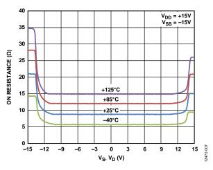
Figure 8. R<sub>ON</sub> as a Function of V<sub>5</sub>, V<sub>D</sub> for Different Temperatures,  $\pm 15$  V Dual Supply
