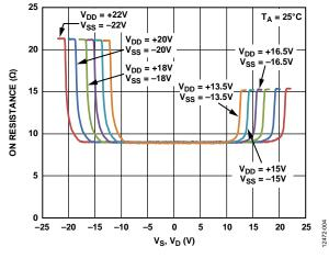
Figure 5. Row as a Function of Vs, VD (Dual Supply)
