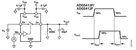
Figure 47. Switching Times, ton and toFF
