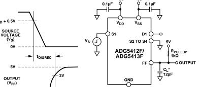
Figure 45. Interrupt Flag Recovery Time,  $t_{DIGREC}$ , with a 1 k $\Omega$  Pull-Up Resistor
