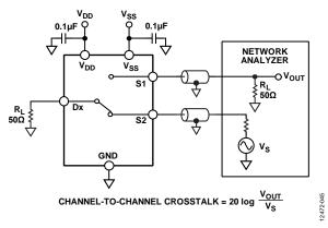
Figure 36. Channel-to-Channel Crosstalk
