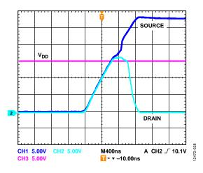
Figure 29. Drain Output Response to Positive Overvoltage
