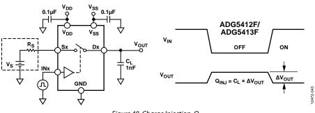
Figure 48. Charge Injection, Q<sub>INJ</sub>
