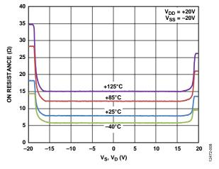
Figure 9.  $R_{ON}$  as a Function of  $V_5$ , $V_D$  for Different Temperatures, ±20 V Dual Supply
