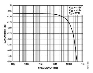
Figure 26. Bandwidth vs. Frequency
