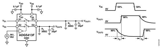
Figure 46. Break-Before-Make Time Delay, t<sub>D</sub>
