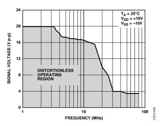
Figure 31. Large Voltage Signal Tracking vs. Frequency
