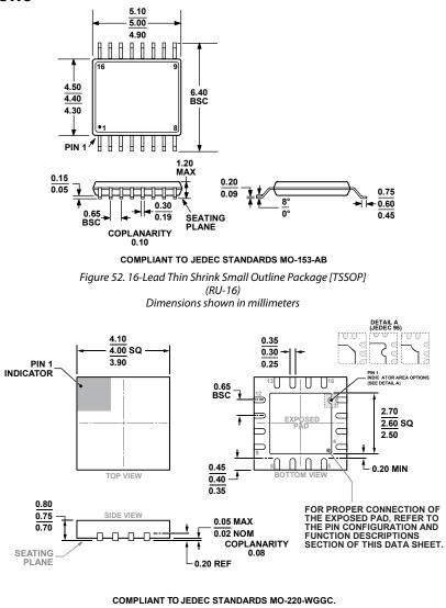
Figure 53.16-Lead Lead Frame Chip Scale Package [LFCSP] 4 mm × 4 mm Body and 0.75 mm Package Height (CP-16-17) Dimensions shown in millimeters
