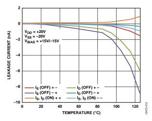
Figure 13. Leakage Current vs. Temperature, ±20 V Dual Supply
