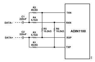
Figure 13. Recommended Hybrid for the ADIN1100
