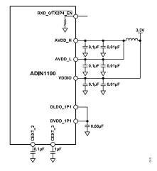
Figure 19. Supplies and Capacitors for Single-Supply 2.4 V p-p Transmit
