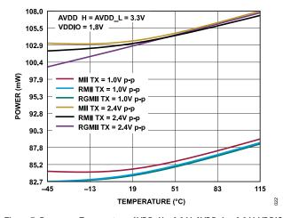
Figure 7. Power vs. Temperature, AVDD\_H = 3.3 V, AVDD\_L = 3.3 V, VDDIO = 1.8 V, Internal LDO Circuit, 10BASE-T1L Mode
