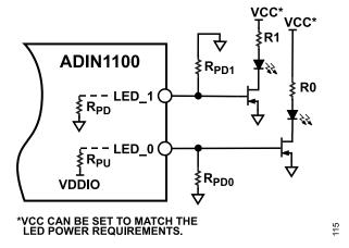
Figure 22. Transistor Controlled LED Configuration
