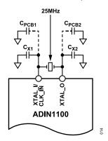
Figure 23. Crystal Oscillator Connection
