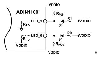
Figure 21. Active Low LED Polarity Configuration
