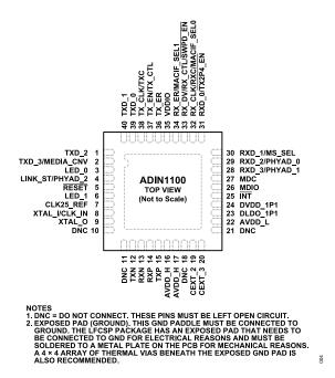
Figure 4. Pin Configuration
