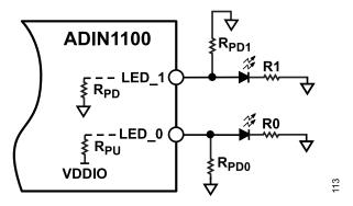
Figure 20. Active High LED Polarity Configuration
