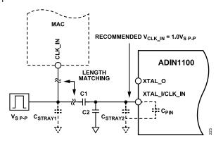
Figure 25. External 50 MHz Clock Input Circuit for RMII Mode
