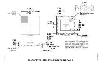
Figure 26. 40-Lead Lead Frame Chip Scale Package [LFCSP] 6 mm × 6 mm Body and 0.75 mm Package Height (CP-40-29) Dimensions shown in millimeters
