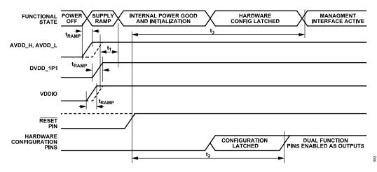
Figure 2. Power-Up Timing
