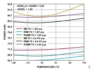
Figure 8. Power vs. Temperature, AVDD\_H = 3.3 V, VDDIO = 3.3 V, AVDD\_L = 1.8 V, Internal LDO Circuit, 10BASE-T1L Mode
