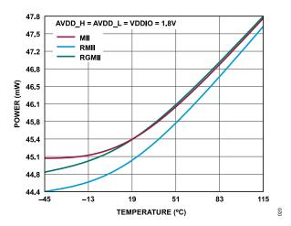
Figure 5. Power vs. Temperature, 1.8 V Single Supply, Internal LDO Circuit, 10BASE-T1L Mode
