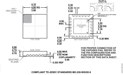
Figure 34. 24-Lead Lead Frame Chip Scale Package [LFCSP] 4 mm × 4 mm Body and 0.75 mm Package Height (CP-24-14) Dimensions shown in millimeters
