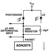
Figure 29. Differential Measurement of IMPD Across a Sense Resistor
