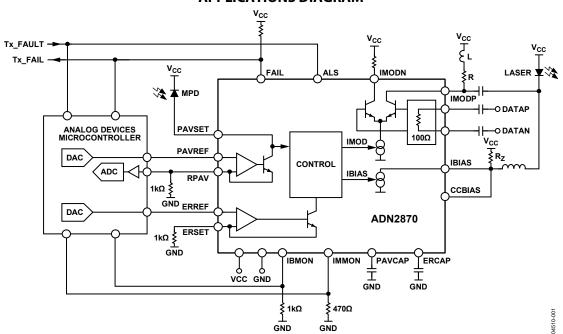
Figure 1. Application Diagram Showing Microcontroller Interface
