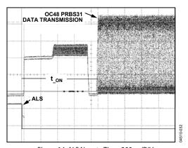
Figure 14. ALS Negate Time, 200 μs/DIV
