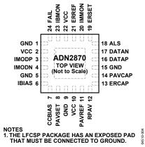
Figure 5. Pin Configuration
