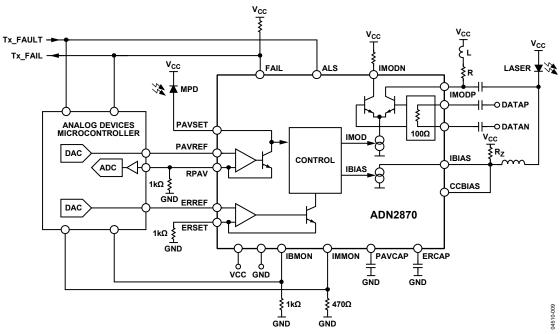
Figure 26. Using MicroConverter Calibration and Monitoring
