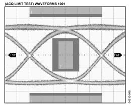
Figure 22. Optical Eye 2.488 Gbps, 65 ps/DIV, PRBS  $2^{31-1}$ , PAV = -0.2 dBm, ER = 8.96 dB, Mask Margin 21%,  $T_A = 85^{\circ}$ C
