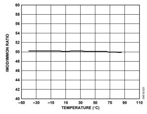
Figure 15. IMOD/IMMON Gain vs. Temperature,  $I_{MOD} = 30 \text{ mA}$
