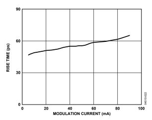
Figure 6. Rise Time vs. Modulation Current, I<sub>BIAS</sub> = 20 mA
