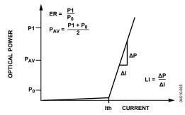
Figure 23. Laser Transfer Function
