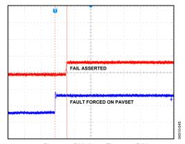
Figure 16. FAIL Assert Time,1 μs/DIV
