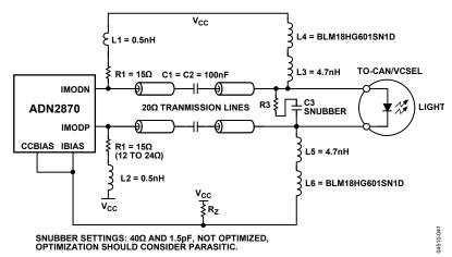
Figure 33. Recommended Differential Drive Circuit
