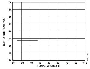
Figure 11. Supply Current (Icc) vs. Temperature with ALS Asserted, IBIAS = 20 mA
