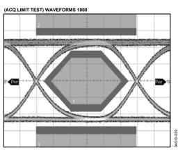
Figure 20. Optical Eye 155 Mbps, 1.078 ns/DIV, PRBS  $2^{31-1}$ , PAV = -4.5 dBm, ER = 9 dB, Mask Margin 50%
