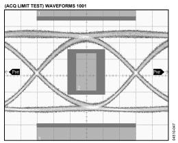
Figure 21. Optical Eye 2.488 Gbps, 65 ps/DIV, PRBS  $2^{31-1}$ , PAV = 0 dBm, ER = 9 dB, Mask Margin 22%,  $T_A = 25^{\circ}$ C
