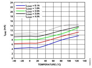
Figure 13. Ground Current ( $I_{GND}$ ) vs. Temperature,  $V_{OUT} = 0.9 V$
