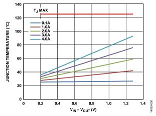
Figure 50. 1000 mm<sup>2</sup> of PCB Copper,  $T_B = 25^{\circ}$ C
