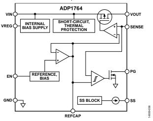
Figure 38. Functional Block Diagram, Fixed Output
