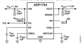
Figure 1. Fixed Output Operation
