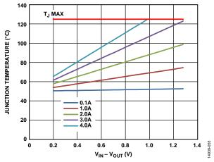
Figure 55. 100 mm<sup>2</sup> of PCB Copper,  $T_B = 50$ °C, LFCSP
