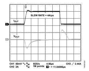
Figure 20. Load Transient Response,  $C_{OUT} = 22 \mu F$ ,  $V_{IN} = 1.8 \text{ V}$ ,  $V_{OUT} = 1.3 \text{ V}$
