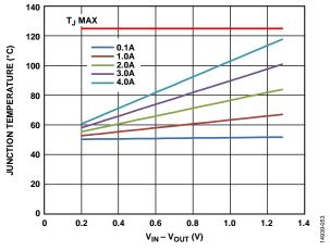
Figure 53. 1000 mm<sup>2</sup> of PCB Copper,  $T_B = 50$ °C, LFCSP
