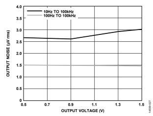
Figure 27. Output Noise vs. Output Voltage (Vouт)
