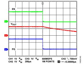
Figure 45.  $V_{OUT}$  vs. Typical PG Voltage Behavior,  $V_{IN}$  Falling ( $V_{OUT} = 1.3 \text{ V}$ )
