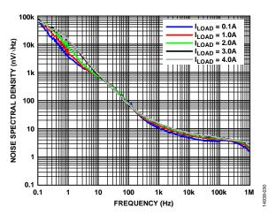
Figure 30. Noise Spectral Density vs. Frequency at Various Load Current (Iout), 0.1 Hz to 1 MHz
