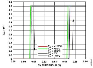
Figure 43. Output Voltage vs. EN Threshold,  $V_{OUT} = 1.3 \text{ V}$
