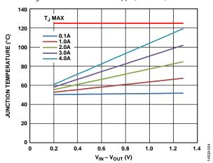
Figure 54. 500 mm<sup>2</sup> of PCB Copper,  $T_B = 50$ °C, LFCSP
