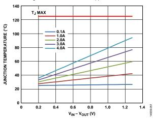
Figure 51. 500 mm<sup>2</sup> of PCB Copper,  $T_B = 25^{\circ}$ C
