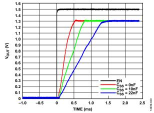
Figure 40. Fixed V<sub>OUT</sub> Ramp-Up with External Soft Start Capacitor (V<sub>OUT,EN</sub>) vs. Time
