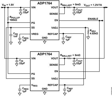
Figure 49. Two ADP1764 Devices Connected in Parallel to Achieve Higher Current Output
