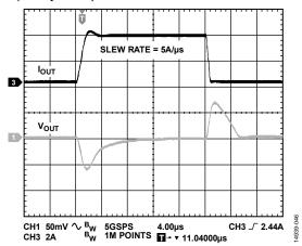
Figure 46. Output Transient Response,  $C_{OUT} = 22 \mu F$ ,  $V_{OUT} = 1.3 V$
