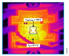
Figure 56. Thermal Image of the ADP1764 Evaluation Board at  $I_{LOAD}$  = 4 A,  $V_{IN}$  = 1.5 V,  $V_{OUT}$  = 1.3 V,  $T_B$  = 91.7°C
