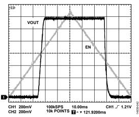
Figure 42. Typical EN Pin Operation
