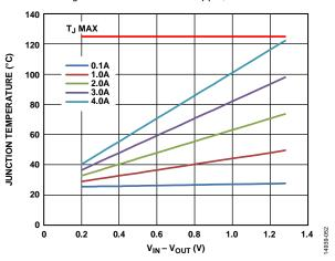
Figure 52. 100 mm<sup>2</sup> of PCB Copper,  $T_B = 25$  °C
