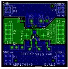
Figure 58. Typical Board Layout, Top Side
