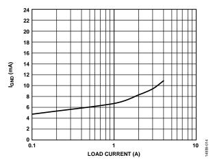
Figure 14. Ground Current (I<sub>GND</sub>) vs. Load Current (I<sub>LOAD</sub>), V<sub>OUT</sub> = 0.9 V
