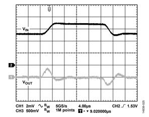
Figure 25. Line Transient Response, Load Current = 4 A,  $V_{IN} = 1.3 \text{ V to } 1.7 \text{ V Step, } V_{OUT} = 0.9 \text{ V}$
