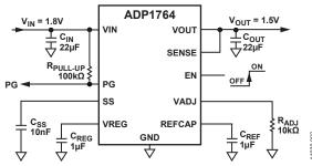
Figure 2. Adjustable Output Operation
