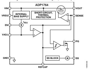
Figure 39. Functional Block Diagram, Adjustable Output
