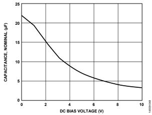
Figure 48. Capacitance vs. DC Bias Voltage
