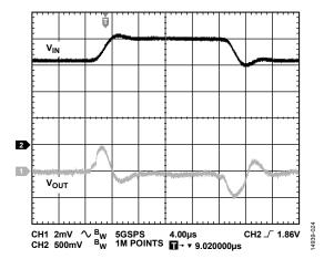
Figure 24. Line Transient Response, Load Current = 4 A,  $V_{IN} = 1.6 \text{ V}$  to 1.98 V Step,  $V_{OUT} = 1.3 \text{ V}$
