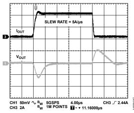
Figure 47. Output Transient Response,  $C_{OUT} = 47 \mu F$ ,  $V_{OUT} = 1.3 V$
