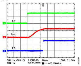
Figure 44. Vout vs. Typical PG Voltage Behavior, V<sub>IN</sub> Rising (Vout = 1.3 V)
