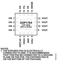
Figure 3. Pin Configuration
