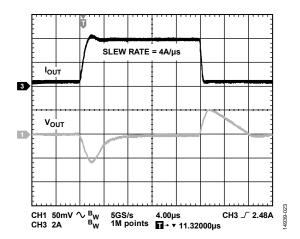
Figure 23. Load Transient Response,  $C_{OUT} = 47 \,\mu\text{F}$ ,  $V_{IN} = 1.4 \,\text{V}$ ,  $V_{OUT} = 0.9 \,\text{V}$
