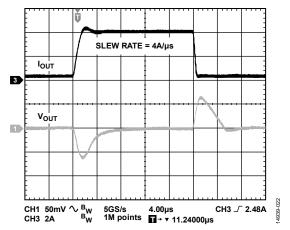
Figure 22. Load Transient Response,  $C_{OUT} = 22 \mu F$ ,  $V_{IN} = 1.4 \text{ V}$ ,  $V_{OUT} = 0.9 \text{ V}$
