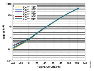
Figure 16. Shutdown Current ( $I_{GND\_SD}$ ) vs. Temperature at Various Input Voltages ( $V_{IN}$ ),  $V_{OUT} = 0.9 \text{ V}$
