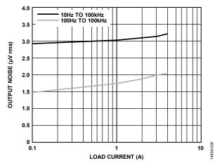
Figure 26. Output Noise vs. Load Current (ILOAD)
