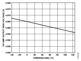
Figure 41. Op Amp Output High Voltage vs. Temperature
