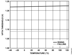
Figure 8. VPTH Threshold vs. Temperature
