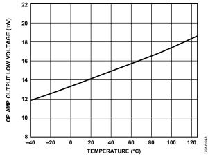
Figure 44. Op Amp Output Low Voltage vs. Temperature
