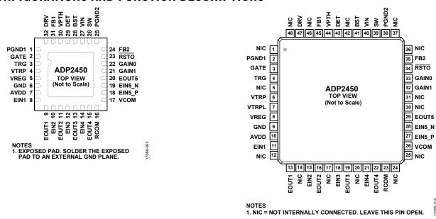
Figure 3. 32-Lead LFCSP Package Pin Configuration (Top View)
