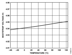
Figure 15. Bootstrap Voltage vs. Temperature
