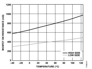
Figure 12. MOSFET On Resistance vs. Temperature
