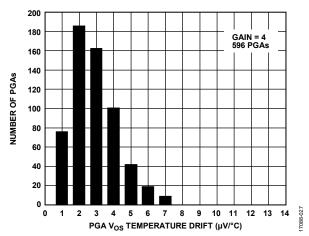
Figure 28. PGA Input Offset Voltage Drift Distribution, Gain = 4
