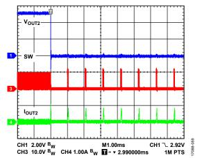
Figure 60. Buck Regulator OCP Triggered
