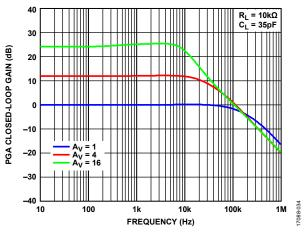
Figure 35. PGA Closed-Loop Gain vs. Frequency
