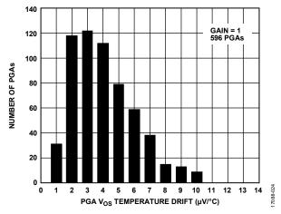
Figure 25. PGA Input Offset Voltage Drift Distribution, Gain = 1
