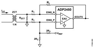
Figure 67. Typical Configuration for Leakage Current Detection
