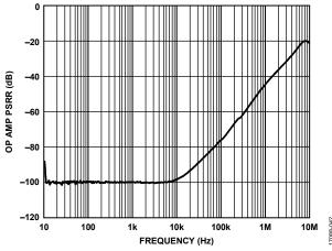
Figure 43. Op Amp PSRR vs. Frequency
