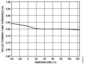
Figure 13. Valley Current-Limit Threshold vs. Temperature
