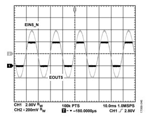
Figure 47. Op Amp No Phase Reversal,  $V_{AVDD} = 4 V$ ,  $A_V = -10$
