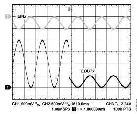
Figure 56. PGA Gain Switching from Gain = 4 to Gain = 1
