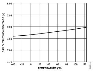
Figure 11. DRV Output High Voltage vs. Temperature
