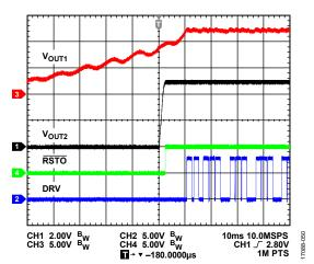
Figure 51. Start Up with AC Current Source, VCOM = GND
