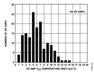
Figure 40. Op Amp Input Offset Voltage Temperature Drift Distribution
