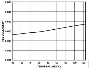
Figure 10. FB2 Voltage vs. Temperature
