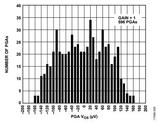
Figure 27. PGA Input Offset Voltage Distribution
