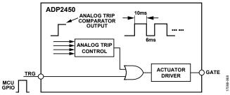
Figure 69. Actuator Driver Control Circuit
