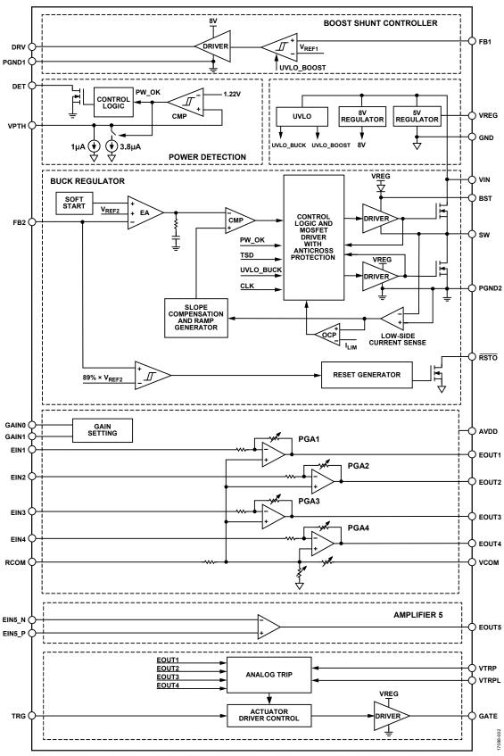
Figure 2. Functional Block Diagram
