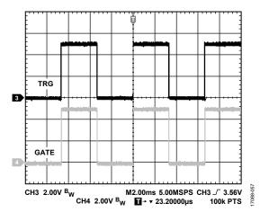
Figure 58. TRG Trigger Analog Trip Function
