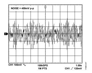
Figure 48. Op Amp 0.1 Hz to 10 Hz Noise, Amplification =  $10,000 \times$
