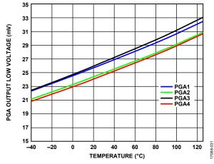
Figure 32. PGA Output Low Voltage vs. Temperature
