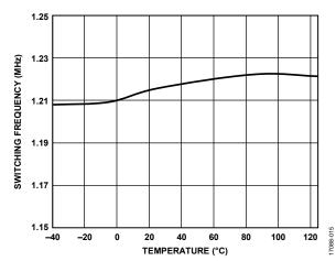
Figure 16. Switching Frequency vs. Temperature
