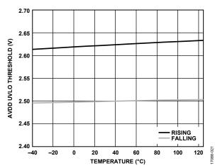
Figure 22. AVDD UVLO Threshold vs. Temperature
