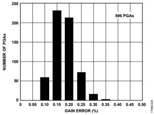
Figure 30. PGA Gain Error Distribution
