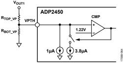
Figure 65. Programmable Voltage of Power Detection
