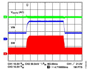
Figure 64. Buck Regulator Line Transient, V<sub>IN</sub> from 8 V to 24 V, Full Load
