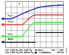
Figure 59. Buck Regulator Soft Start with Full Load  $(V_{OUT2} = 3.3 V, Adjustable Version)$
