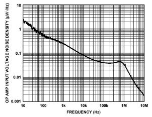
Figure 50. Op Amp Input Voltage Noise Density vs. Frequency
