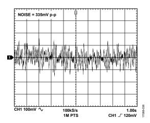
Figure 39. PGA 0.1 Hz to 10 Hz Noise, Amplification =  $10,000 \times$
