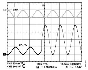
Figure 53. PGA Gain Switching from Gain = 1 to Gain = 4
