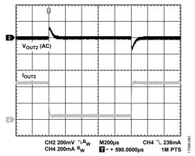
Figure 61. Buck Regulator Load Transient (50 mA to 450 mA)
