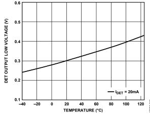
Figure 14. DET Output Low Voltage vs. Temperature
