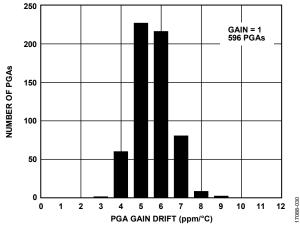
Figure 31. PGA Gain Drift Distribution, Gain = 1
