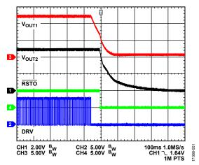
Figure 52. System Shutdown Waveform
