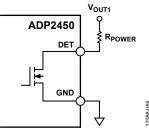
Figure 66. Dummy Load Connection
