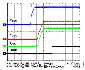
Figure 62. Buck Regulator Soft Start with Full Load  $(V_{OUT2} = 5 V, Fixed Version)$
