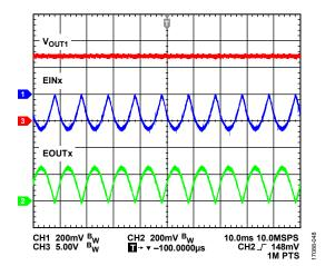
Figure 49. PGA Working Waveform, Gain = 1
