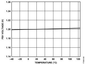
Figure 7. FB1 Voltage vs. Temperature
