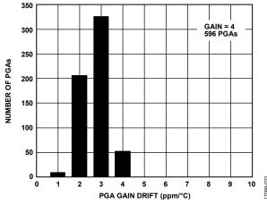
Figure 34. PGA Gain Drift Distribution, Gain = 4
