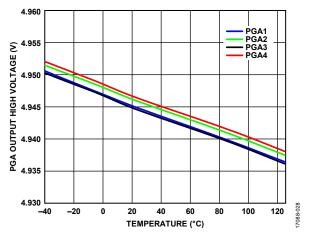
Figure 29. PGA Output High Voltage vs. Temperature
