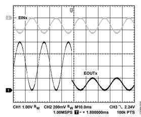
Figure 57. PGA Gain Switching from Gain = 16 to Gain = 4
