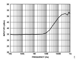
Figure 16. Input IP3 vs. Frequency (Low Frequency Detail)
