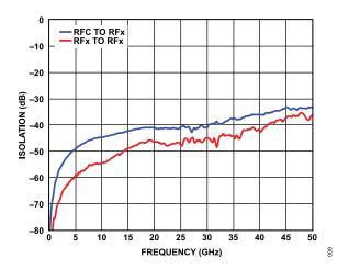
Figure 11. Isolation vs. Frequency with Impedance Match
