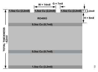
Figure 22. Probe Matrix Board (Cross Section View)
