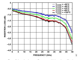
Figure 7. Insertion Loss vs. Frequency with Impedance Match
