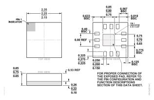
Figure 26. 12-Terminal Land Grid Array [LGA]
