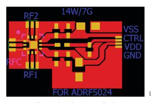
Figure 23. Probe Board Layout (Top View)
