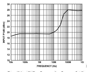
Figure 15. Input P1dB vs. Frequency (Low Frequency Detail)
