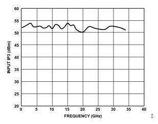
Figure 14. Input IP3 vs. Frequency
