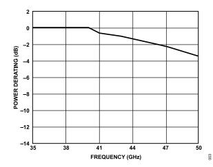
Figure 3. Power Derating vs. Frequency, High Frequency Detail, T<sub>CASE</sub> = 85°C
