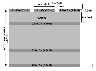
Figure 17. Evaluation Board (Cross Section View)
