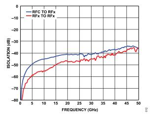
Figure 12. Isolation vs. Frequency Without Impedance Match
