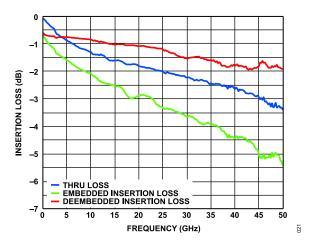
Figure 19. Insertion Loss vs. Frequency
