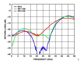
Figure 10. Return Loss vs. Frequency for RFC and RFx (On) Without Impedance Match
