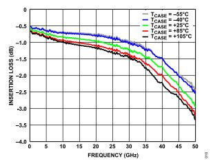
Figure 9. Insertion Loss vs. Frequency Without Impedance Match
