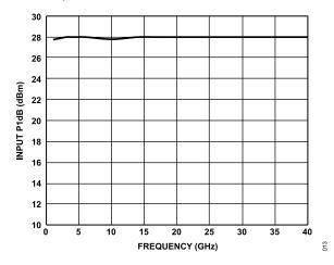
Figure 13. Input P1dB vs. Frequency
