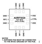
Figure 4. Pin Configuration (Top View)
