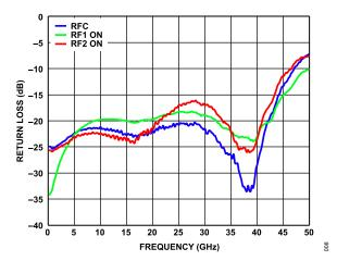
Figure 8. Return Loss vs. Frequency for RFC and RFx (On) with Impedance
