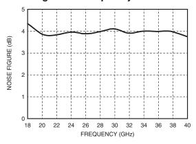
Note: Measured Performance Characteristics (Typical Performance at 25°C) Vd1 = 5V, Id1 = 45 mA
