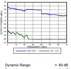
Resolution:0.1 dBPower Accuracy: $\pm 1 \text{ dB} > 500 \text{ MHz}$  $\pm 2 \text{ dB} \le 500 \text{ MHz}$  $\pm 2 \text{ dB} \le -20 \text{ dBm}$  (All Frequencies)RF OFF< -90 dBm
