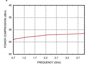
P0.1dB Vs. Frequency @ VDD= 5V  $T_A = +25^{\circ} \text{ C}$
