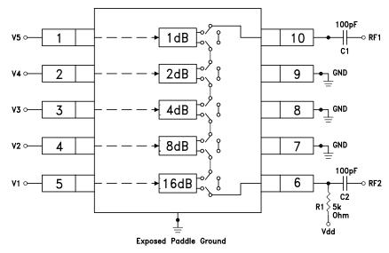
DC blocking capacitors C1 & C2 are required on RF1 & RF2. Choose C1 =  $C2 = 100 \sim 300$  pF to allow lowest customer specific frequency to pass with minimal loss. R1 = 5K Ohm is required to supply voltage to the circuit through either PIN 6 or PIN 10.
