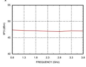
Input IP3 vs. Frequency @ VDD= 5V,  $T_A = +25^{\circ}$  C
