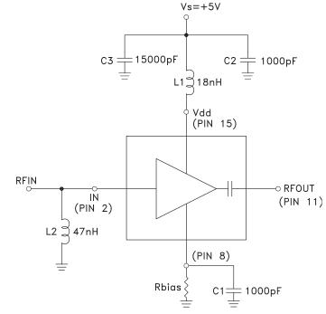
Note 1: L1, L2 and C1 should be located as close to the pins as possible.
