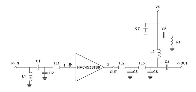
Note: C2 and C3 should be placed as close to pins as possible.
