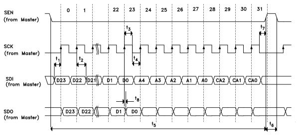
Figure 5. SPI Timing Diagram
