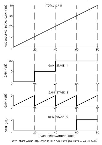
Figure 4. Decode Logic Gain Allocation
