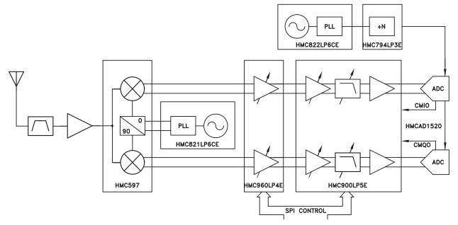
Figure 1. Typical Receive Path Block Diagram Showing HMC960LP4E
