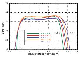
Figure 16. Output IP3 vs. Output Common Mode, High Linearity Bias Settings [3][6]
