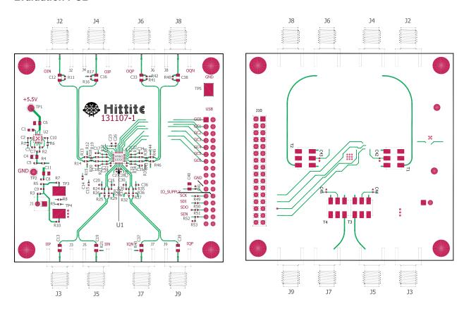
The circuit board used in the application should use RF circuit design techniques. Signal lines should have 50 Ohms impedance while the package ground leads and exposed paddle should be connected directly to the ground plane similar to that shown. A sufficient number of via holes should be used to connect the top and bottom ground planes. The evaluation circuit board shown is available from Hittite upon request.
