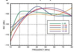
Figure 8. Output IP2 vs. Frequency & Gain [4]
