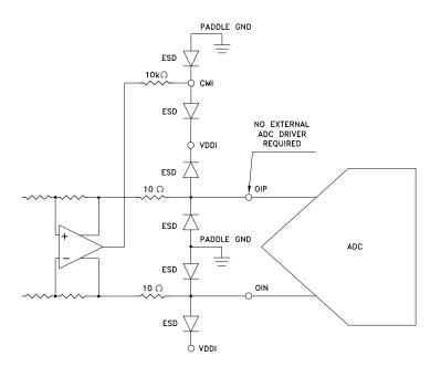
Figure 3. Output Driver Block Diagram
