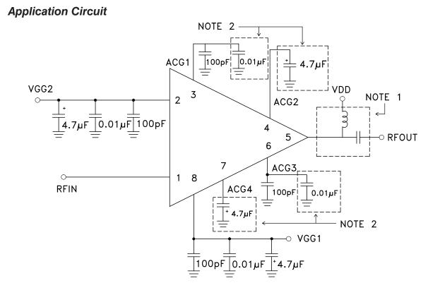
NOTE 1: Drain Bias (Vdd) must be applied through a broadband bias tee with low series resistance and capable of providing 500 mA.
