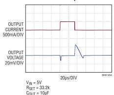
V<sub>IN</sub> = 5V R<sub>SET</sub> = 33.2k C<sub>OUT</sub> = 10μF C<sub>SET</sub> = 0.47μF LOAD STEP = 10mA TO 500mA
