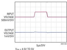
$$\begin{split} &V_{|N} = 4.5 V \text{ TO 5V} \\ &R_{SET} = 33.2 k \\ &C_{OUT} = 10 \mu F \\ &C_{SET} = 0.47 \mu F \\ &I_{\perp} = 500 \text{mA} \end{split}$$
