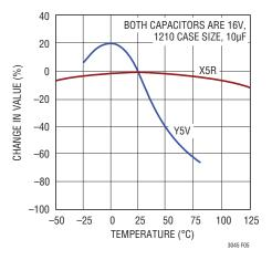
Figure 5. Ceramic Capacitor Temperature Characteristics
