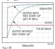
$R_{SET} = 33.2k$   $C_{OUT} = 10\mu F$   $C_{SET} = 4.7\mu F$   $R_{L} = 6.6\Omega$
