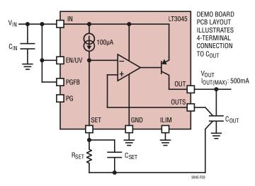
Figure 3.  $C_{OUT}$  and  $C_{SET}$  Connections for Best Performance
