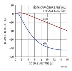
Figure 4. Ceramic Capacitor DC Bias Characteristics
