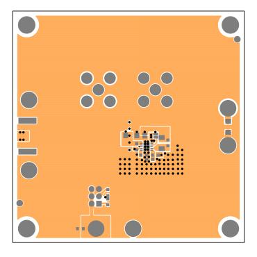
Figure 8. Recommended DFN Layout
