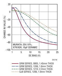
Figure 6. Capacitor Voltage Coefficient for Different Case Sizes
