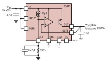
Figure 1. Basic Adjustable Regulator
