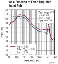
**Power Supply Ripple Rejection**
