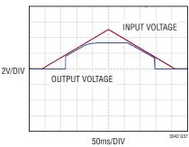
V<sub>IN</sub> = 0V TO 5V  $\begin{aligned} &V_{EN/UV} = V_{IN} \\ &R_{SET} = 33.2k \\ &C_{OUT} = 10 \mu F \\ &C_{SET} = 0.47 \mu F \\ &R_L = 6.6 \Omega \end{aligned}$
