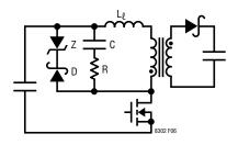
Figure 6. (RC + DZ) Snubber Circuit
