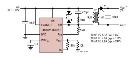
3V to 32V<sub>IN</sub>/5V<sub>OUT</sub> Isolated Flyback Converter
