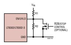
Figure 7. Undervoltage Lockout (UVLO)
