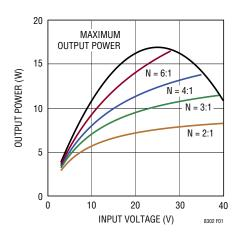
Figure 1. Output Power for 3.3V Output
