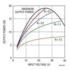
Figure 3. Output Power for 12V Output
