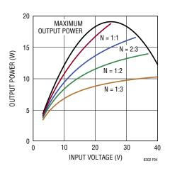
Figure 4. Output Power for 24V Output
