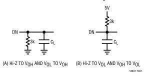
**Load Circuits for Output Float Delay**
