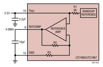
Figure 4a. LTC1867 Reference Circuit
