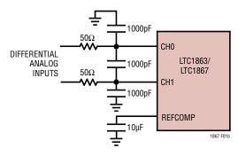
Figure 1b. Optional RC Input Filtering for Differential Inputs
