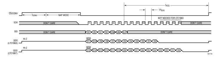
Figure 6. Example 1,  $\overline{\text{CS}}/\text{CONV}$  Starts a Conversion and Remains HIGH Until Next Data Transfer. With  $\overline{\text{CS}}/\text{CONV}$  Remaining HIGH After the Conversion, Automatic Nap Modes Provides Power Reduction at Reduced Sample Rate.
