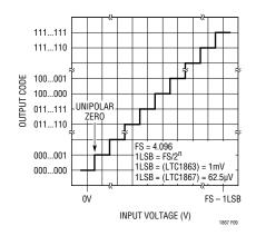
Figure 9. LTC1863/LTC1867 Unipolar Transfer Characteristics (Straight Binary)
