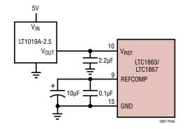
Figure 4b. Using the LT1019-2.5 as an External Reference
