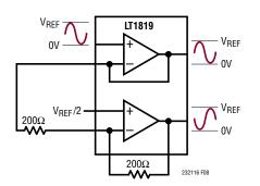
Figure 8. Single-Ended to Differential Driver
