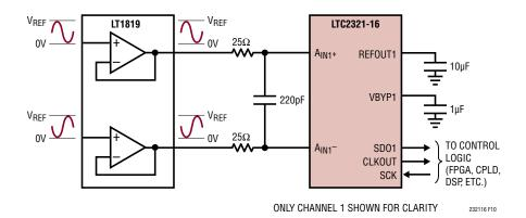
Figure 10. Fully-Differential Application Circuit
