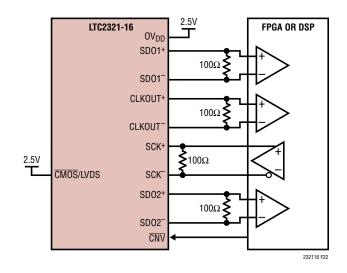
Figure 22. LTC2321 Using the LVDS Interface
