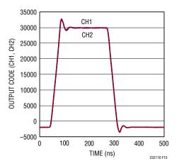
Figure 15. Transient Response of the LTC2321-16
