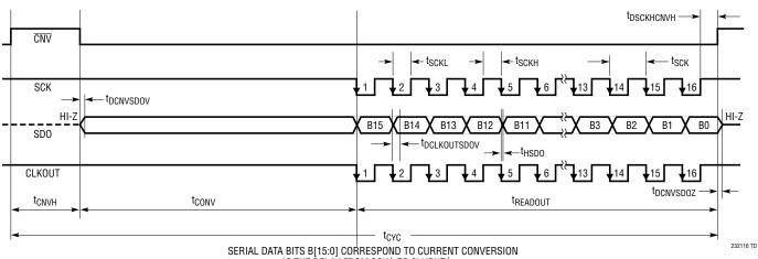
$t_{DSCKCLKOUT}$  IS THE DELAY FROM SCK  $\downarrow$  TO CLKOUT  $\downarrow$
