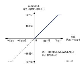
Figure 7. Pseudo-Differential Unipolar Transfer Function
