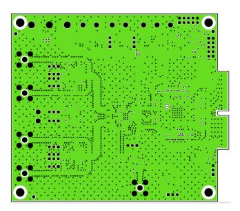
Figure 24. Layer 2, Ground Plane
