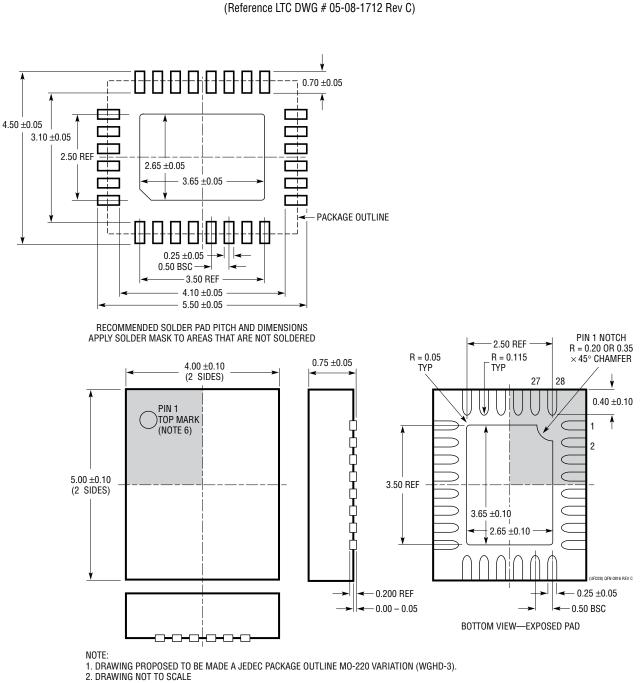
**UFD** Package 28-Lead Plastic QFN (4mm × 5mm)
