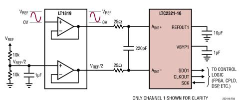
Figure 4. Pseudo-Differential Bipolar Application Circuit
