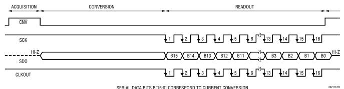
SERIAL DATA BITS B[15:0] CORRESPOND TO CURRENT CONVERSION
