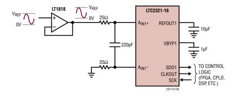
Figure 6. Pseudo-Differential Unipolar Application Circuit
