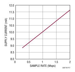
Figure 17. Power Supply Current of the LTC2321-16 Versus Sampling Rate
