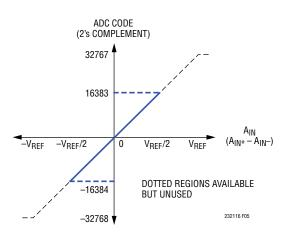
Figure 5. Pseudo-Differential Bipolar Transfer Function
