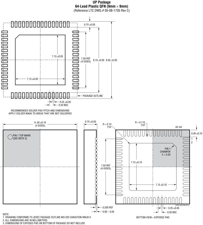
3. DIMENSIONS OF EXPOSED PAD ON BOTTOM OF PACKAGE DO NOT INCLODE MOLD FLASH. MOLD FLASH, IF PRESENT, SHALL NOT EXCEED 0.20mm ON ANY SIDE, IF PRESENT
