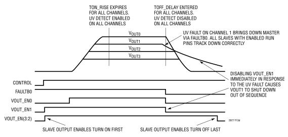
Figure 13d. Improperly Configured Fault Response on Faulting Channel Disrupts Tracking
