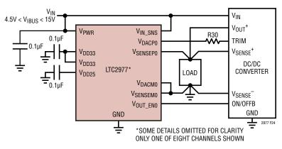
Figure 24. Application Circuit for DC/DC Converters with Trim Pin
