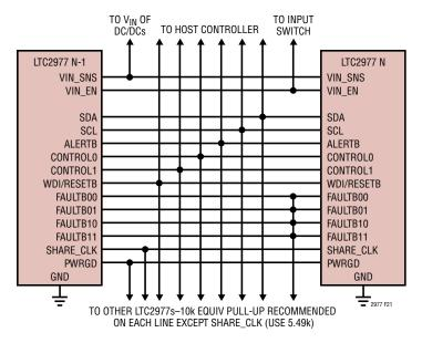
Figure 21. Typical Connections Between Multiple LTC2977s
