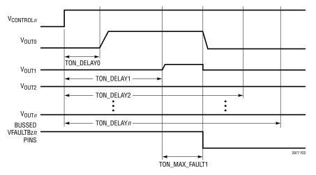
Figure 22. Aborted On Sequence Due to Channel 1 Short
