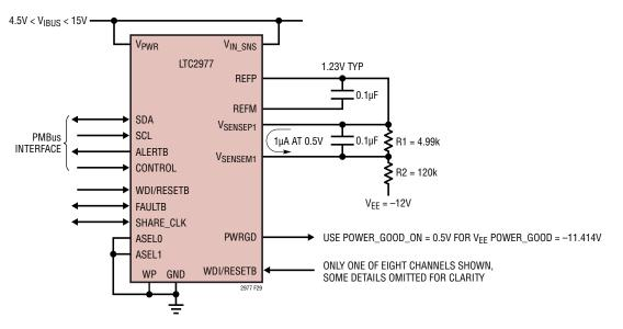
Figure 29. Sensing Negative Voltages
