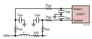
Figure 26. Inductor DCR Current Sensing Circuits
