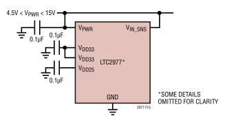
Figure 15. Powering LT2977 Directly from an Intermediate Bus
