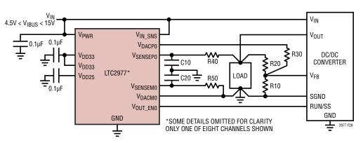
Figure 28. Anti-Aliasing Filter on V<sub>SENSE</sub> Lines
