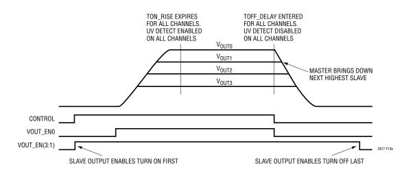
Figure 13b. Control Pin Tracking All Supplies Up And Down
