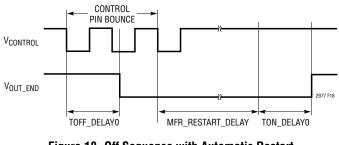
Figure 18. Off Sequence with Automatic Restart
