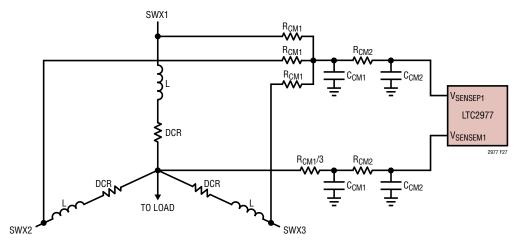
Figure 27. Multiphase DCR Current Sensing Circuits
