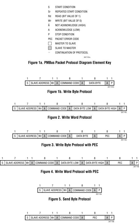
Figure 6. Send Byte Protocol with PEC
