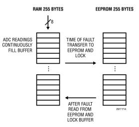
Figure 14. Fault Log Conceptual Diagram
