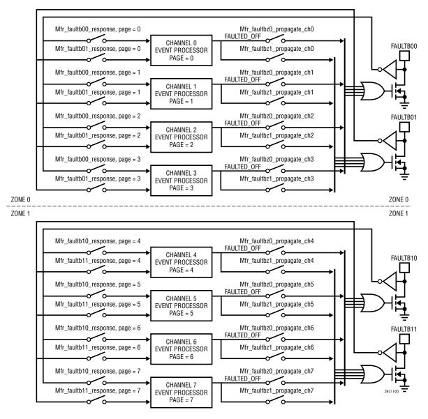
Figure 20. Channel Fault Management Block Diagram
