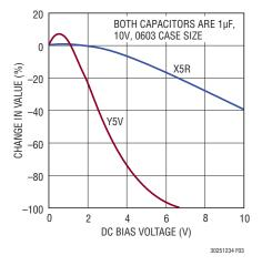
Figure 3. Ceramic Capacitor DC Bias Characteristics
