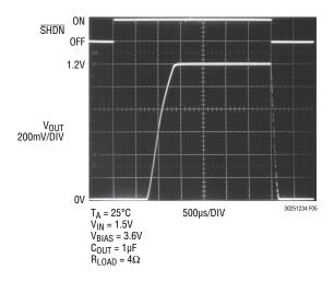
Figure 5. Output Start-Up and Shutdown
