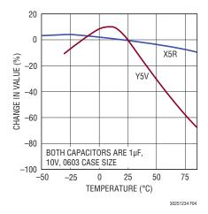
Figure 4. Ceramic Capacitor Temperature Characteristics
