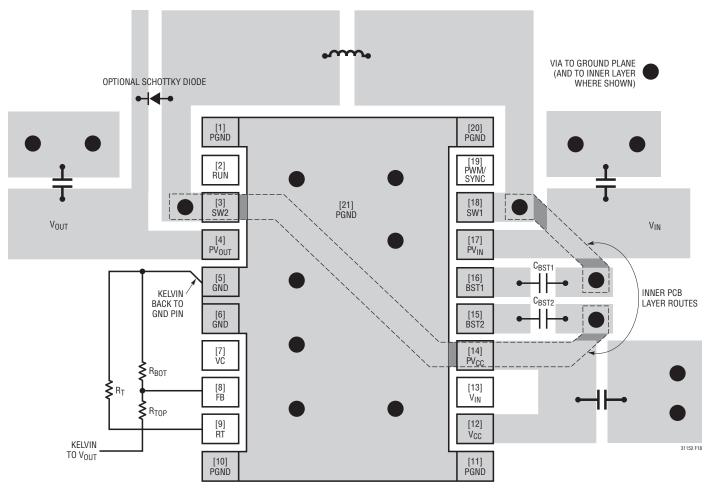
UNINTERRUPTED GROUND PLANE SHOULD EXIST UNDER ALL COMPONENTS SHOWN IN BOLD AND UNDER TRACES CONNECTING TO THOSE COMPONENTS
