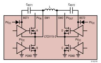
Figure 1. Power Stage Schematic
