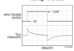
OA to 2A Load Step,  $V_{IN} = 13.8V$
