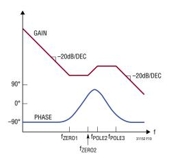
Figure 10. Type III Compensation Bode Plot
