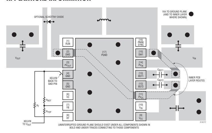
Figure 17. PCB Layout Recommended for the DHD Package
