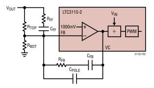
Figure 2. Error Amplifier and Compensation Network
