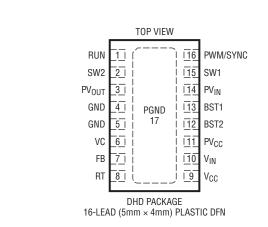
$T_{JMAX}$  = 125°C,  $\theta_{JA}$  = 43°C/W,  $\theta_{JC}$  = 4.3°C/W EXPOSED PAD (PIN 17) IS PGND, MUST BE SOLDERED TO PCB
