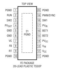
$T_{JMAX}$  = 150°C,  $\Theta_{JA}$  = 38°C/W,  $\Theta_{JC}$  = 10°C/W EXPOSED PAD (PIN 21) IS PGND, MUST BE SOLDERED TO PCB FOR RATED THERMAL PERFORMANCE
