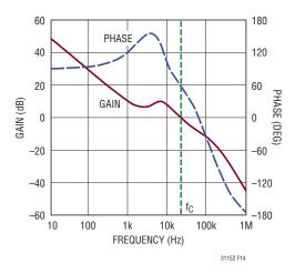
Figure 14. Complete Loop Bode Plot
