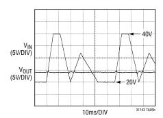
0A to 1.5A Load Step,  $V_{IN} = 20V$
