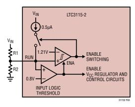
Figure 3. Accurate RUN Pin Comparator
