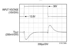
Fast (10 $\mu$ s) Cold Crank Line Transient,  $V_{IN}=13.8V$  to 4V
