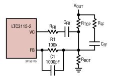
Figure 15. R1 and C1 are Recommended if  $R_{T0P}$  <  $1 M\Omega$
