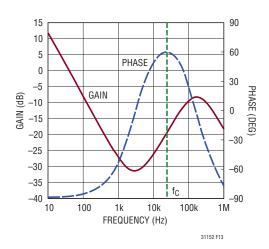
Figure 13. Compensated Error Amplifier Bode Plot
