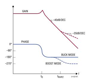
Figure 7. Buck-Boost Converter Bode Plot
