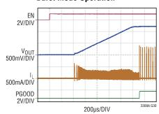
$3.3V_{IN}$  to  $1.2V_{OUT}, 2MHz$  Typical Application  $R_{LOAD}=120\Omega$
