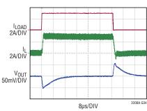
$3.3V_{IN}$  to  $1.2V_{OUT}, 2MHz$  Typical Application  $C_{OUT}=44\mu F,~L=330nH$  LOAD STEP: 50mA TO 3A ( $10A/\mu s)$
