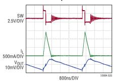
$3.3V_{IN}\,$  to  $1.2V_{OUT},\,2MHz$  Typical Application  $C_{OUT}$  =  $44\mu F,\,\,L$  =  $330nH,\,\,I_{LOAD}$  = 100mA
