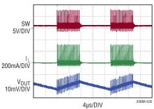
5.0V<sub>IN</sub> to 1.2V<sub>OUT</sub>, 2MHz Application  $C_{OUT} = 44\mu F$ , L = 330nH,  $I_{LOAD} = 2mA$
