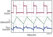
$3.3V_{|N}$  to  $1.2V_{OUT},$  2MHz Typical Application  $C_{OUT}=44\mu F,~L=330nH,~I_{LOAD}{=}500mA$
