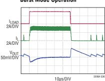
$3.3V_{IN}$  to  $1.2V_{OUT},$  2MHz Typical Application  $C_{OUT}=44\mu F,~L=330nH$  LOAD STEP: 50mA TO 3A (10A/ $\mu s$ )
