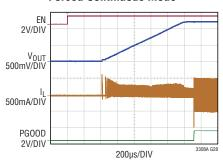
$3.3 V_{|N}~$  to  $1.2 V_{OUT}, 2 MHz$  Typical Application  $R_{LOAD} = 120 \Omega$
