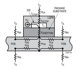
Figure 4. Multi-Laver PCB with Thermal Vias Acts as a Heat Sink
