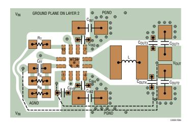
(b) With Capacitors  $C_{OUT1}$  and  $C_{OUT2}$  Rotated by 90°, Which Reduces High Frequency Output Ripple. Optional 0201 Capacitors  $C_{OUT3}$  and  $C_{OUT4}$  Further Improve the High Frequency Output Ripple. Five 5mil Vias Are Used within the EPAD. For Layouts Where 5mil Vias Are Not Allowed, It Is Recommended to Use Either Four 8mil Vias or a Single (Filled or Tented) 12mil Diameter Via.
