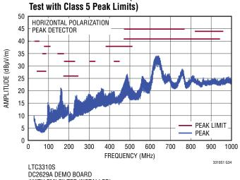
DC2629A DEMO BOARD (WITH EMI FILTER INSTALLED) 3.3V INPUT TO 1.2V OUTPUT AT 7.5A, f<sub>SW</sub> = 2MHz
