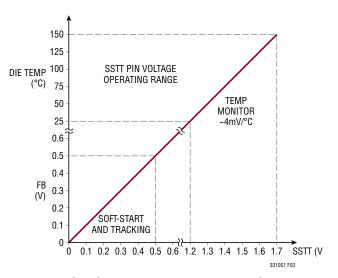
Figure 3. Soft-Start and Temperature Monitor Operation
