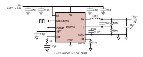
LTC3310S, High Efficiency, 2MHz, 0.5V, 10A, Pulse Skip, Low Part Count
