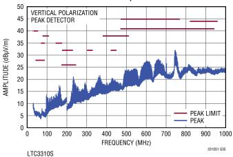
LIC3310S DC2629A DEMO BOARD (WITH EMI FILTER INSTALLED) 3.3V INPUT TO 1.2V OUTPUT AT 7.5A, f<sub>SW</sub> = 2MHz
