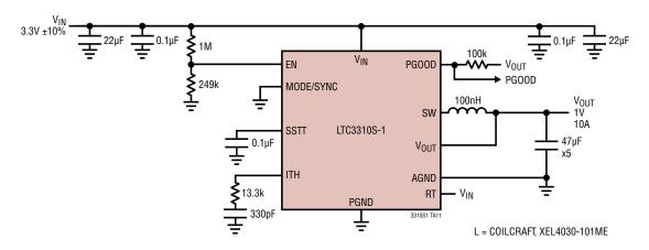
LTC3310-1, 2MHz, 1.0V, Forced Continuous 1.5A DC to 7.5A Step Load 6A/µs Transient, <3% Total Variation
