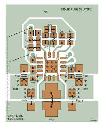
Figure 5. Recommended PCB Layout for the LTC3310
