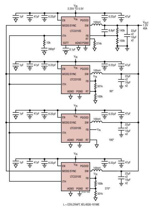
Four Phase, 2MHz, 1.2V, 40A Driven with External Clock
