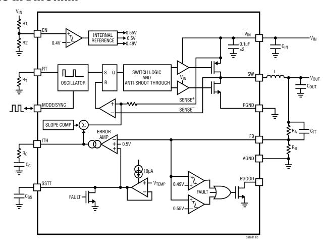
Note 1: On the LTC3310S-1 the  $R_{\mbox{\scriptsize A}}$  and  $R_{\mbox{\scriptsize B}}$  resistors are internal.
