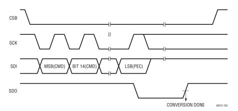
Figure 33. SDO Polling Using PLADC Command (Parallel Configuration)
