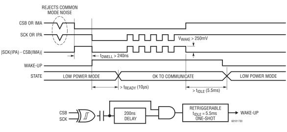
Figure 30. Wake-up Detection and IDLE Timer
