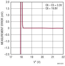
Measurement Error Due to a V<sup>+</sup> AC Disturbance
