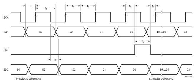
Figure 22. Timing Diagram of 4-Wire Serial Peripheral Interface
