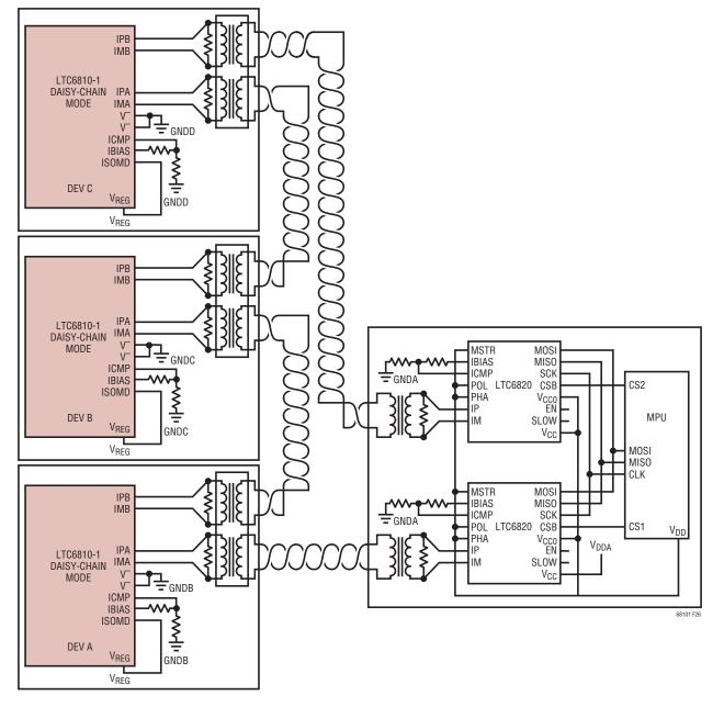
Figure 26. Reversible isoSPI Daisy Chain using the LTC6810-1
