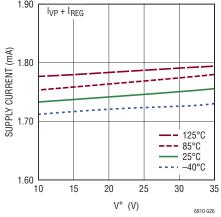
Standby Supply Current vs V<sup>+</sup> Internal REG Enabled
