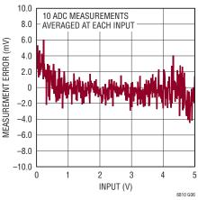
Measurement Noise vs Input **Fast Mode**
