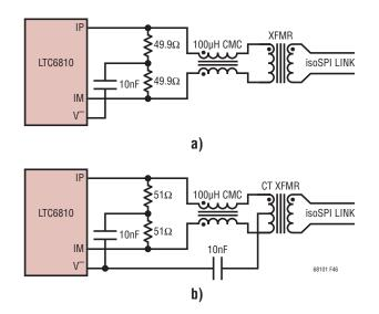
Figure 46. Daisy Chain Interface Components
