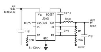
Figure 37.  $V_{\text{REG}}$  Powered from Cell Stack with High Efficiency Regulator
