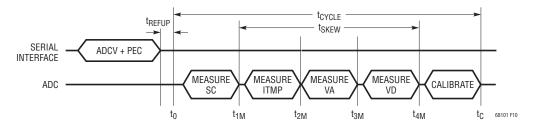
Figure 10. Timing for ADSTAT command measuring SC, ITMP, VA, VD
