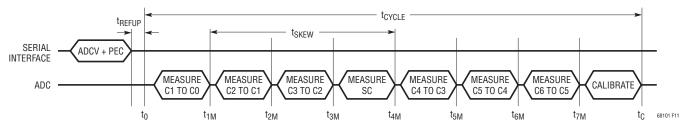
Figure 11. Timing for ADCVSC Command, SCONV = 0
