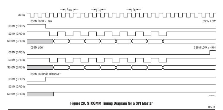
signal is sent, the SDA and SCL lines are held high and all data in the rest of the word is ignored. If ICOMn[3:0] is a NO TRANSMIT, both SDA and SCL lines are released, and rest of the data in the word is ignored. This is used when a particular device in the stack does not have to communicate to a slave.
