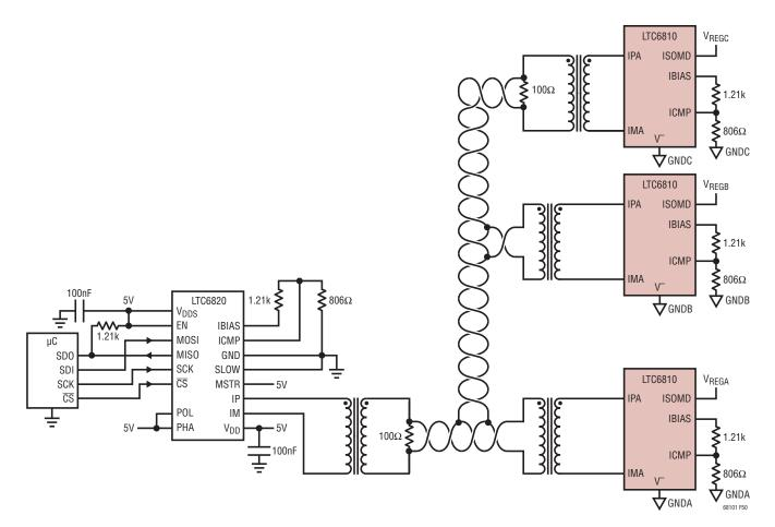
Figure 50. Connecting the LTC6810-2 in a Multi-Drop Configuration
