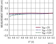
Measurement Error vs Common Mode Voltage
