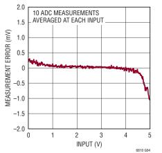
**Measurement Noise vs Input Normal Mode**
