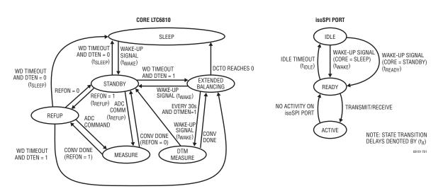
Figure 1. LTC6810 Operation State Diagram
