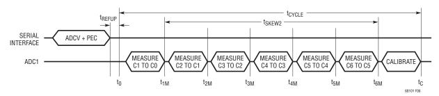
Figure 6. Timing for ADCV Command Measuring All 6 Cells, SCONV = 0
