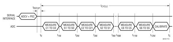
Figure 12. Timing for ADCV Command Measuring All 6 Cells, SCONV = 1
