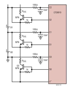
Figure 41. External Discharge Circuit
