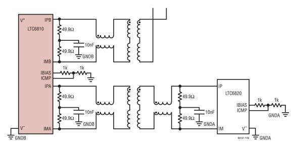
Figure 49. Interfacing an LTC6810-1 with a  $\mu C$  Using an LTC6820 for Isolated SPI Control
