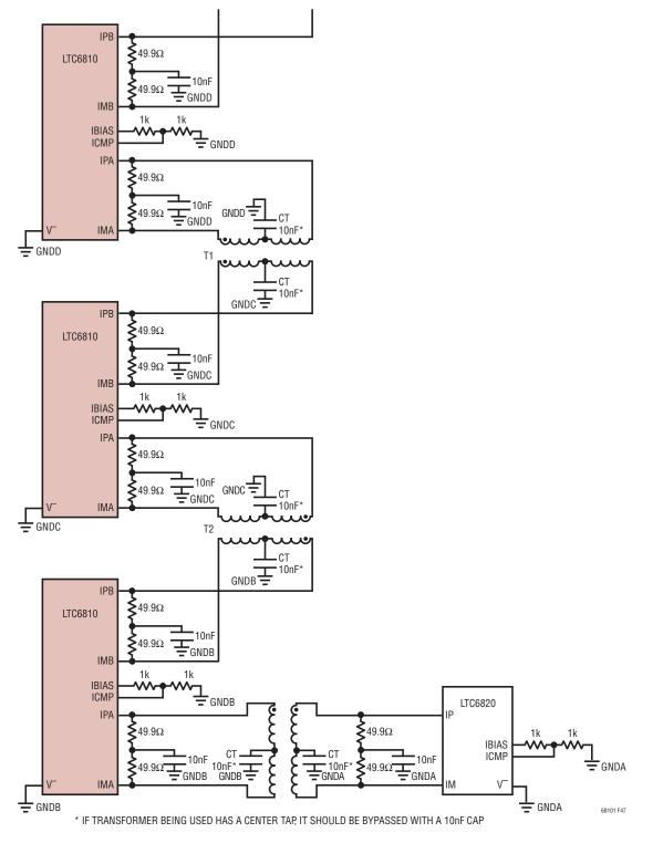
Figure 47. Daisy Chain Interface Components on Single Board
