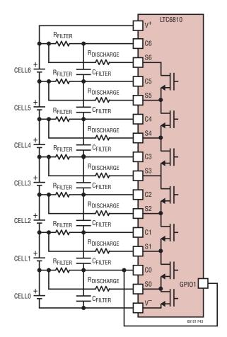
Figure 42. Seven Cell with Internal Discharge
