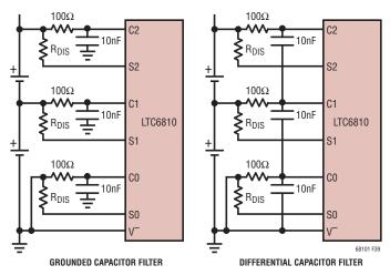
Figure 39. Input Filter Structure Configurations
