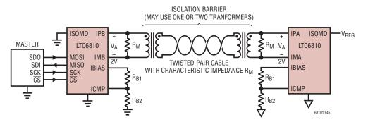
Figure 44. isoSPI Circuit
