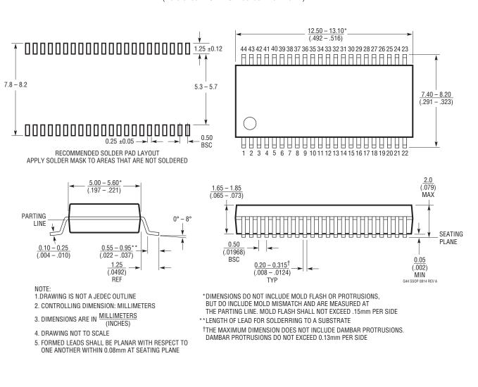
G Package 44-Lead Plastic SSOP (5.3mm) (Reference LTC DWG # 05-08-1754 Rev A)
