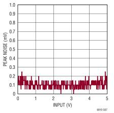
**Measurement Error vs Input Filtered Mode**
