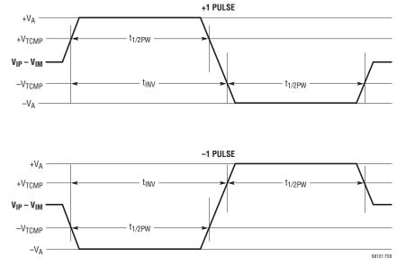
Figure 28. isoSPI Pulse Detail
