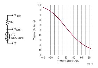
Figure 53. Typical Temperature Probe Circuit and Relative Output
