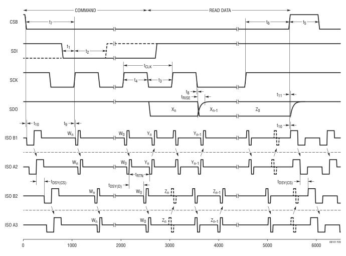
Figure 29. isoSPI Timing Diagram
