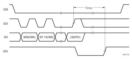
Figure 32. SDO Polling After an ADC Conversion Command (Parallel Configuration)
