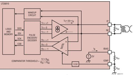
Figure 23. isoSPI Interface
