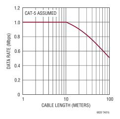
Figure 45. Data Rate vs Cable Length
