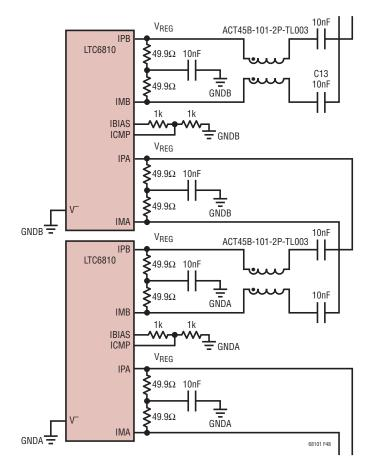
Figure 48. Capacitive Isolation Coupling for LTC6810-1s on the Same PCB
