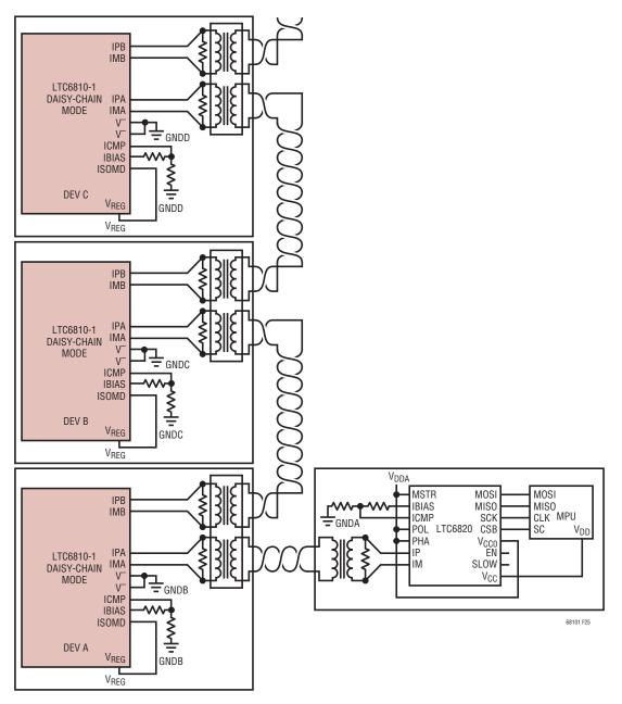
Figure 25. Transformer-Coupled Daisy-Chain Configuration Using LT6810-1
