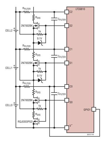
Figure 43. Seven Cell with External Discharge
