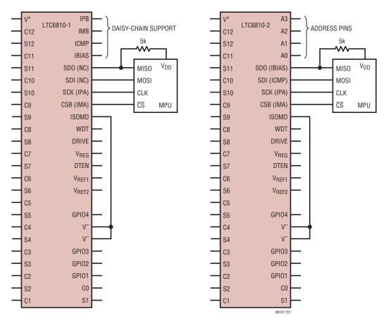
Figure 21. 4-Wire SPI Configuration
