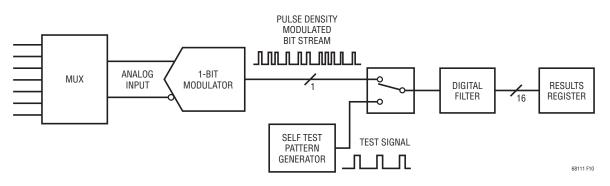
Figure 16. Operation of LT6810 ADC Self Test
