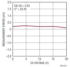
Measurement Error Due to a V<sub>REG</sub>
