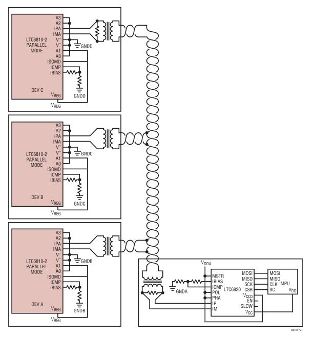
Figure 27. Transformer-Coupled Multi-Drop Configuration Using LT6810-2
