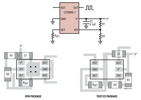
Figure 22. Supply Bypassing and PCB Layout
