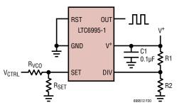
Figure 20. Voltage-Controlled Oscillator
