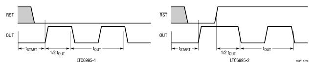
Figure 9. Start-Up Timing Diagram (Reset = 0, POL Bit = 1)
