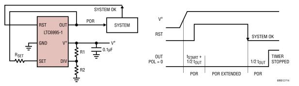
Figure 14. Extended POR. Timer Reset During Initial POR Interval. Full POR Interval Provided Once System Signals the OK
