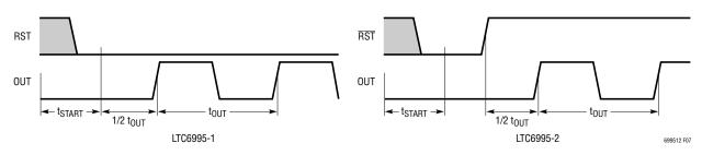
Figure 7. Start-Up Timing Diagram (Reset = 0, POL Bit = 0)
