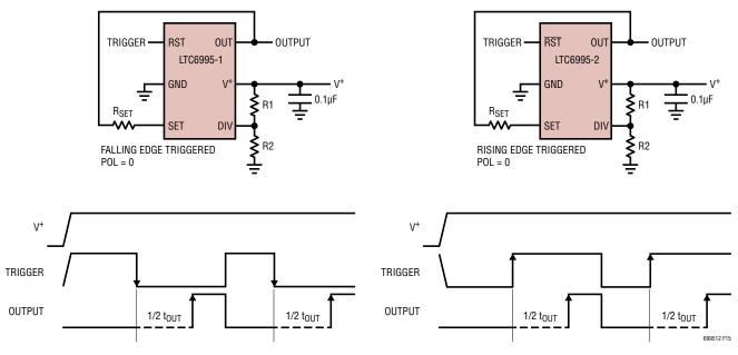
Figure 15. Long Time Delayed Rising Edge. Delay Time Can Range from 500µs to 4.8 Hours
