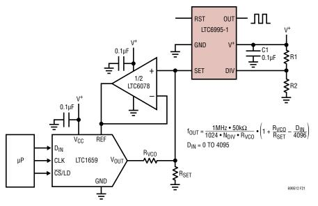
Figure 21. Digitally-Controlled Oscillator
