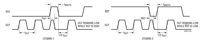
Figure 3. Reset Timing Diagram (POL Bit = 0)
