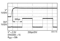
Figure 6. Typical Start-Up LTC6995-1 with RST = 0V
