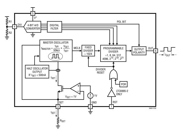
The LTC6995 is built around a master oscillator with a 1MHz maximum frequency. The oscillator is controlled by the SET pin current ( $I_{SET}$ ) and voltage ( $V_{SET}$ ), with a 1MHz • 50k conversion factor that is accurate to ±0.8% under typical conditions.
