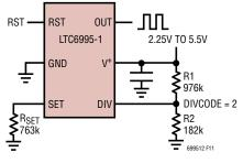
Figure 11. 1Hz Oscillator
