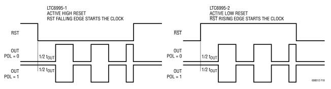
Figure 18. Gated Oscillators. First One-Half Cycle Time Always Accurate
