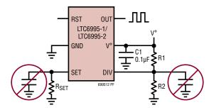
**RST or RST (Pin 4/Pin 1):** Output Reset. The reset input is used to stop the output oscillator and to clear internal dividers. When reset is released the oscillator starts with a full half period time interval. The output logic state when reset is determined by the programmed DIVCODE. The LTC6995-1 has an active high RST input. The LTC6995-2 has an active low RST input.
