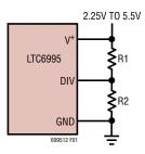
Figure 1. Simple Technique for Setting DIVCODE
