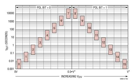
Figure 2. Frequency Range and POL Bit vs DIVCODE
