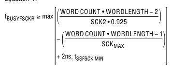
where  $t_{BUSYFSCKR}$  is the time between the falling edge of BUSY and the 1st rising edge of SCK, SCK2 is the nominal configured frequency in Hz and SCK\_MAX is the maximum frequency in Hz.
