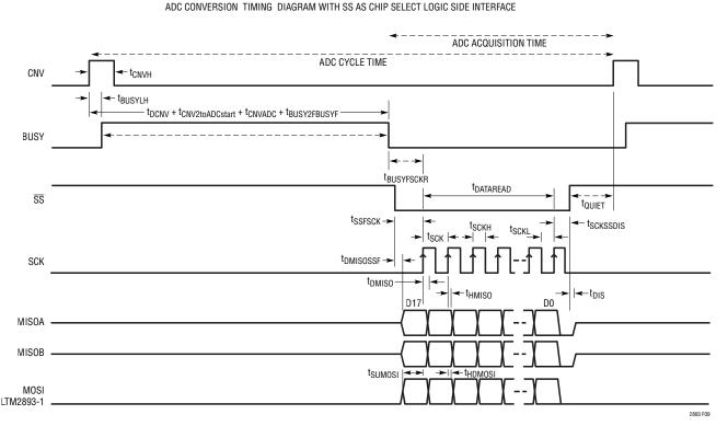
Figure 9. Logic Side Interface of ADC
