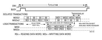
Figure 5. LTM2893-1 Worst Case Example Word Delay on Isolated Transactions When Logic Side Reads and Writes After a Long Delay
