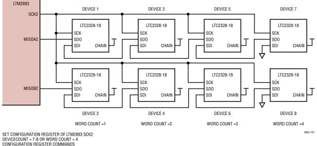
0x10h, 0x9Eh (66MHz, 24-BITS) or 0x10h, 0x94h (66MHz, 18-BITS)
