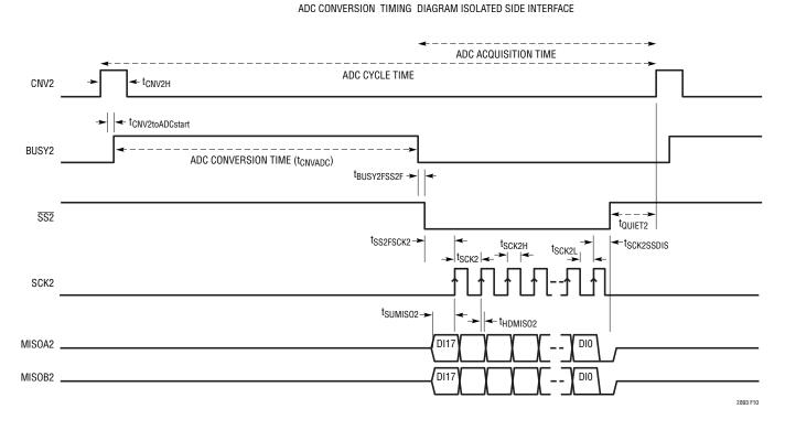
Figure 10. Isolated Side Interface for an ADC Conversion
