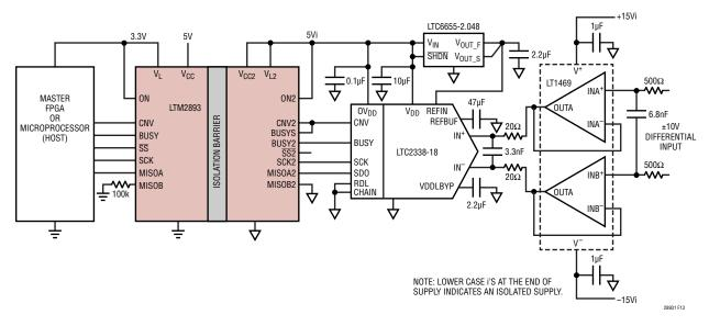
Figure 13. Isolated 1Msps LTC2338-18 Fully Differential ±10V Input Range, with ADC Sleep Disabled (CNV2 = BUSYS)
