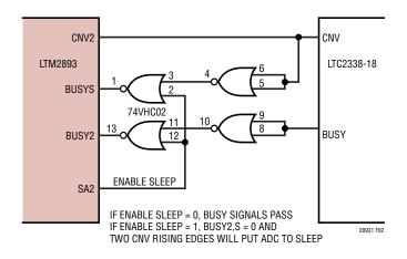
Figure 2. ADC Keep-Alive and Sleep Enable
