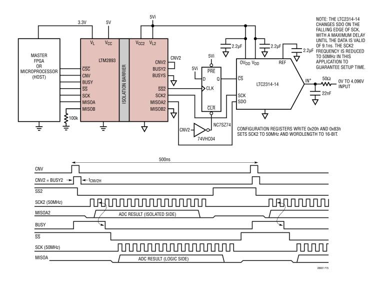
Figure 15. Isolated 2Msps LTC2314-14 OV to 4.096V Input Range, ADC Without a CNV or BUSY, LTC2314  $\overline{\text{CS}}$  Is Synchronized to Low Jitter CNV2
