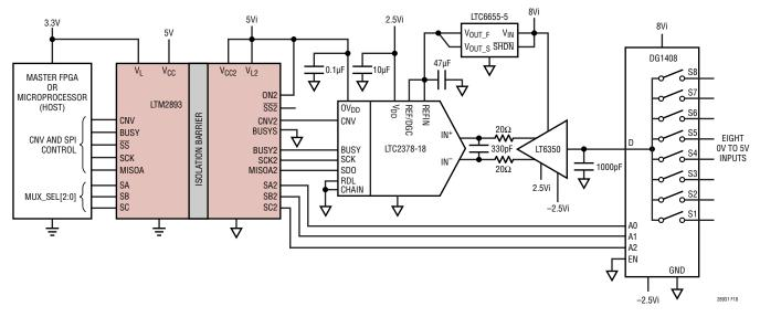
Figure 18. Use of SA, SB, SC Pins for Multiplexing Analog Inputs to ADC
