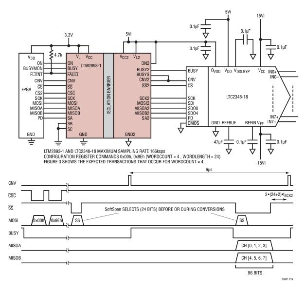
Figure 19. LTM2893-1 with SoftSpan™ Configurable LTC2348-18 8-Channel Simultaneous Sampling ADC
