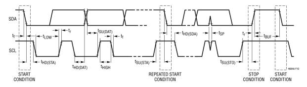
Figure 10. PMBus Timing Diagram
