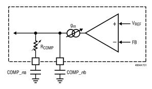
Figure 31. Programmable Loop Compensation
