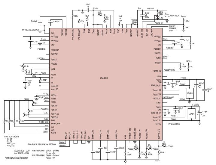
Figure 47. 54V to 1.0V at 30A and 1.5V Outputs at 25A With Providing I<sup>2</sup>C/SMBus/PMBus Serial Interface
