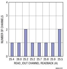
READ\_IOUT of 16 LTM4664A Channels  $12V_{IN}$ ,  $1V_{OUT}$ ,  $T_J = 25^{\circ}C$ ,  $I_{OUTn} = 25A$ , System Having Reached Thermally Steady-State Condition, No Airflow
