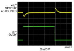
48V TO 1V DUAL PHASE SINGLE OUTPUT, 0A TO 25A/µs LOAD STEP C<sub>0UT</sub> = 470µF ×2 POSCAP, 5 × 330µF CER, COMP\_C0,1 = 1500pF, COMP\_C01b = 100pF, EA-GM = 4.36ms, RCOMP = 13k, PSM FREQ = 350kHz, I<sub>LIMIT</sub> RANGE = LOW V<sub>0UT</sub> RANGE = LOW
