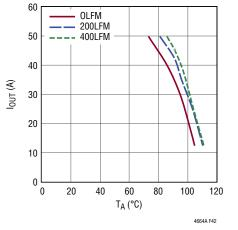
Figure 42. LTM4664A 54V<sub>IN</sub> 1V<sub>OUT</sub> Derating Curve No Heat Sink
