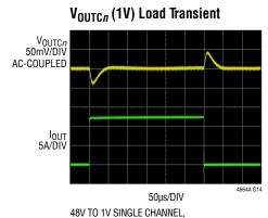
40V TO TV SINGLE CHAINVEL, OA TO 12.5A/µS LOAD STEP  $C_{OUT} = 470 \mu F \times 2 \text{ POSCAP}, 100 \mu F \times 5 \text{ CER},$ COMP\_Cna = 2200 pF, COMP\_Cnb = 100 pF, EA-GM = 3.69 ms, RCOMP = 5k, PSM FREQ = 250 kHz, I<sub>LIMIT</sub> RANGE = LOW V<sub>OUT</sub> RANGE = LOW
