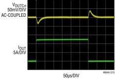
48V TO 1.5V SINGLE CHANNEL, 0A TO 12.5A/ $\mu$ s LOAD STEP C<sub>0UT</sub> = 470 $\mu$ F ×1 POSCAP, 330 $\mu$ F ×2 CER, COMP\_C*n*a = 2200PF, COMP\_C*n*b = 220PF, EA-GM = 3.02ms, RCOMP = 6k, PSM FREQ = 350kHz
