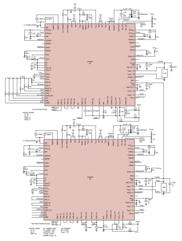
Figure 50. 48V-58V Input, Converting 1.2V at 30A, and 0.9V at 90A. Power System Management Features Accessible Through LTM4664A Over 2-Wire I<sup>2</sup>C/SMBus/PMBus Serial Interface.
