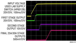
48V TO 1V AT 0A LOAD, EACH 25A/30A STAGE FINAL STAGE TON DELAY AND TON RISE SET TO 100ms
