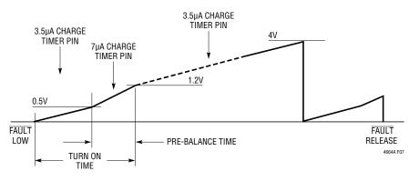
Figure 7. Timer Behavior During Fault or Startup
