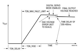
Figure 29. Timing Controlled V<sub>OUT</sub> Rise
