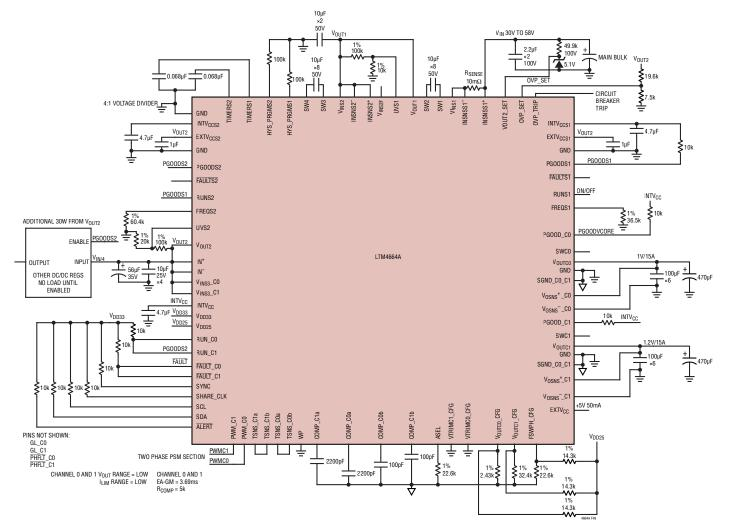
Figure 49. 30V – 58V to 1V and 1.2V at 15A, with Additional 30W from V<sub>OUT2</sub>. Integrated Power System Management Features Accessible Over 2-Wire I<sup>2</sup>C/SMBus/PMBus Serial Interface. For Evaluation and More Information, See Demo Boards DC2143
