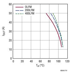
Figure 41. LTM4664A 48V<sub>IN</sub> 1V<sub>OUT</sub> Derating Curve No Heat Sink
