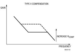
Figure 33. R<sub>COMP</sub> Adjust
