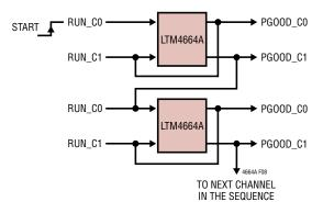
Figure 8. Event (Voltage) Based Sequencing
