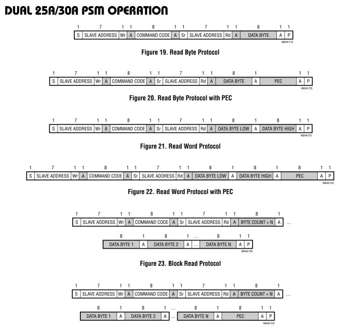
Figure 24. Block Read Protocol with PEC
