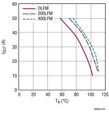
Figure 44. LTM4664A 54V<sub>IN</sub> 1.5V<sub>OUT</sub> 350kHz Derating Curve No Heat Sink
