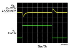
48V TO 0.9V DUAL PHASE SINGLE OUTPUT, 0A TO 25A/µs LOAD STEP  $C_{OUT} = 470\mu$ F ×2 POSCAP, 330µF ×5 CER, COMP\_C0, 1 = 1500pF, COMP\_C01b = 100pF, EA-GM = 4.36ms, RCOMP = 13k, PSM FRED = 250kHz, I<sub>LIMIT</sub> RANGE = LOW V<sub>OUT</sub> RANGE = LOW
