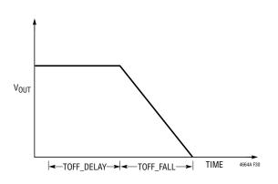
Figure 30. TOFF\_DELAY and TOFF\_FALL
