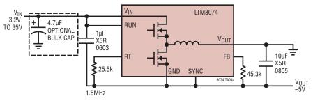
PINS NOT USED IN THIS CIRCUIT: TR/SS, PG
