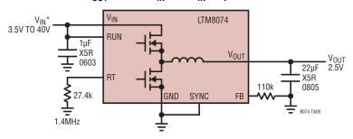
PINS NOT USED IN THIS CIRCUIT: TR/SS, PG  $^{\star}\mathrm{V}_{\mathrm{IN}}$  MAY BE AS LOW AS 3.2V WITH OFF-CYCLE SKIPPING
