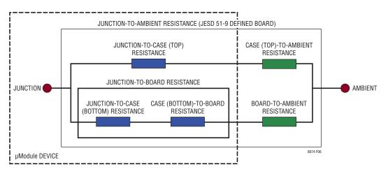
Figure 6. Simplified Graphical Representation of the Thermal Resistance Between the Device Junction and Ambient
