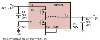
PINS NOT USED IN THIS CIRCUIT: TR/SS, PG
