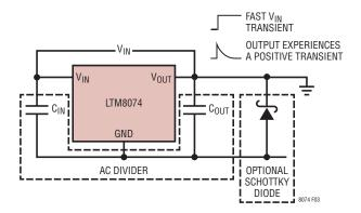
Figure 3. A Schottky Diode Can Limit the Transient Caused by a Fast Rising  $V_{\text{IN}}$  to Safe Levels
