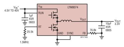
PINS NOT USED IN THIS CIRCUIT: TR/SS, PG  $^{\star}\mathrm{V}_{IN}$  MAY BE AS LOW AS 3.6V WITH OFF-CYCLE SKIPPING
