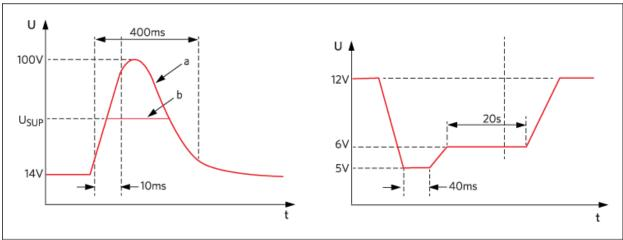
Figure 3. The nominal  $12V_{DC}$  battery supply is actually a complex and somewhat hostile electrical rail, as shown by these voltage vs. time characterizations of a) load-dump surge, and b) cold-crank voltage.
