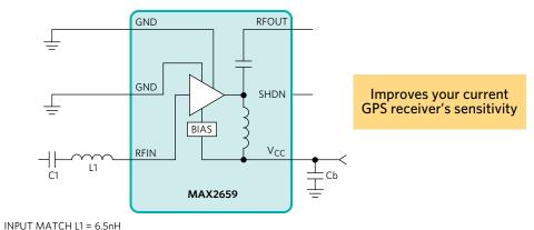
INPUT DC BLOCK C1 = 1800pF SUPPLY BYPASS Cb = 33nF
