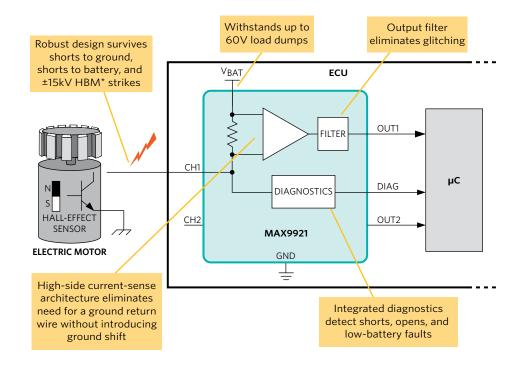
Ideal for window lifters (antipinch control), magnetic relays, automatic doors, seatbelt buckles, electric sunroofs, and powered liftgate controllers
