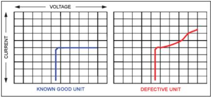
Figure 4. Semiconductor curve tracer plots for the circuit in Figure 3. Curve tracer current/div.is 50μA; voltage/div. is 1V.
