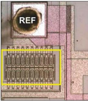
Figure 2A. A circuit in visible light shows no apparent damage from EOS or ESD. The liquid crystal area (marked in yellow) of the circuit is damaged by heat.
