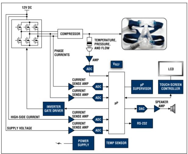
Functional block diagram of a CPAP system. For a list of Maxim's recommended solutions for CPAP designs, please go to: www.maximintegrated.com/CPAP.
