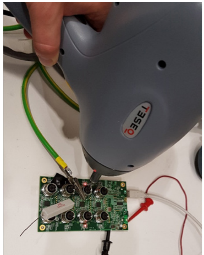
Figure 39. ESD Testing of MAX14819
