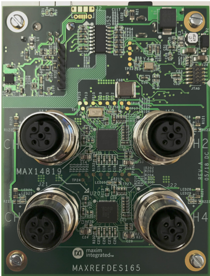
Figure 26. MAXREFDES165 4-Port IO-Link Master Reference Design
