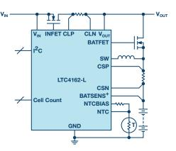
Figure 2. The application circuit for LTC4162 is as simple as it gets for a fullfeatured switching battery charger.
