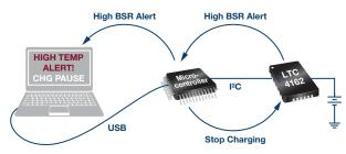
Figure 3. The LTC4162's integrated telemetry system will fulfill almost any monitoring and alert requirements.
