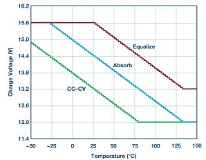
Figure 5. Default 12 V lead-acid temperature profile.
