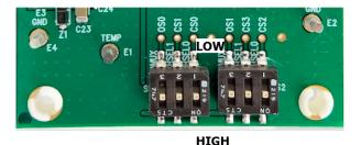
Figure 3. DC2900 Switch Positions for High and Low
