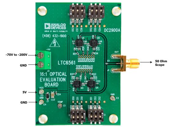
Figure 1. DC2900A Connection Diagram
