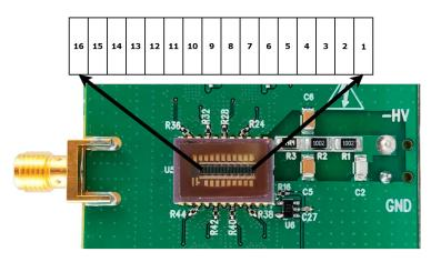
Figure 4. APD Channel Orientation
