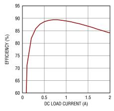
Figure 3. Efficiency vs. Load Current at  $V_{IN}$  = 3.3V,  $V_{OUT1}$  = 1.2V,  $f_{SW}$  = 2MHz
