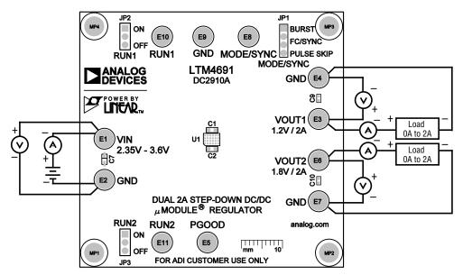
Figure 1. Proper Measurement Equipment Setup
