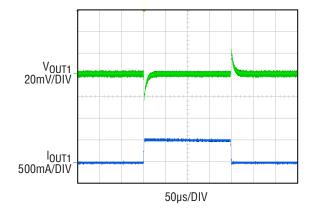
Figure 7. Load Step at  $V_{IN}$  = 3.3V,  $V_{OUT1}$  = 1.2V,  $f_{SW}$  = 2MHz
