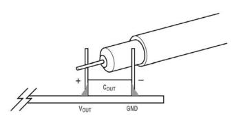
Figure 2. Measuring Output Voltage Ripple
