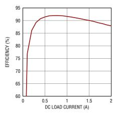
Figure 4. Efficiency vs. Load Current at  $V_{IN}$  = 3.3V,  $V_{OUT2}$  = 1.8V,  $f_{SW}$  = 2MHz
