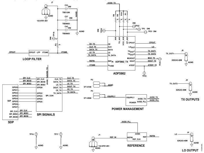
Figure 6. EV-ADF5902SD1Z Evaluation Board Schematic (Page 1)
