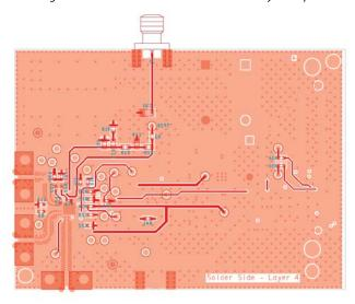
Figure 14. EV-ADF5902SD1Z Evaluation Board Layer 4 Bottom Side
