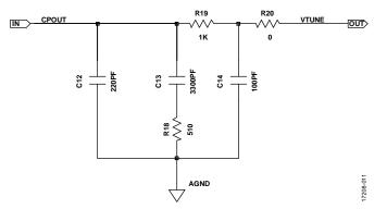
Figure 11. EV-ADF5902SD1Z Evaluation Board Schematic (Page 6)
