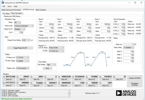
Figure 5. PLL Software Window Display, ADF5902 Ramps Generation
