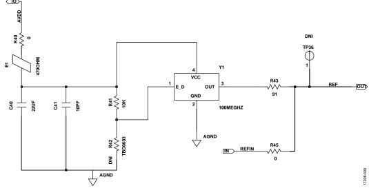
Figure 9. EV-ADF5902SD1Z Evaluation Board Schematic (Page 4)
