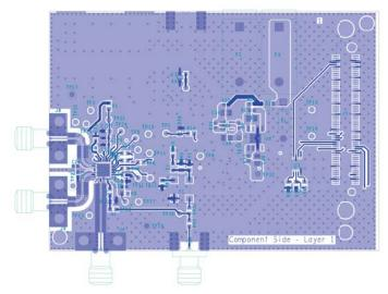
Figure 13. EV-ADF5902SD1Z Evaluation Board Layer 1 Top Side
