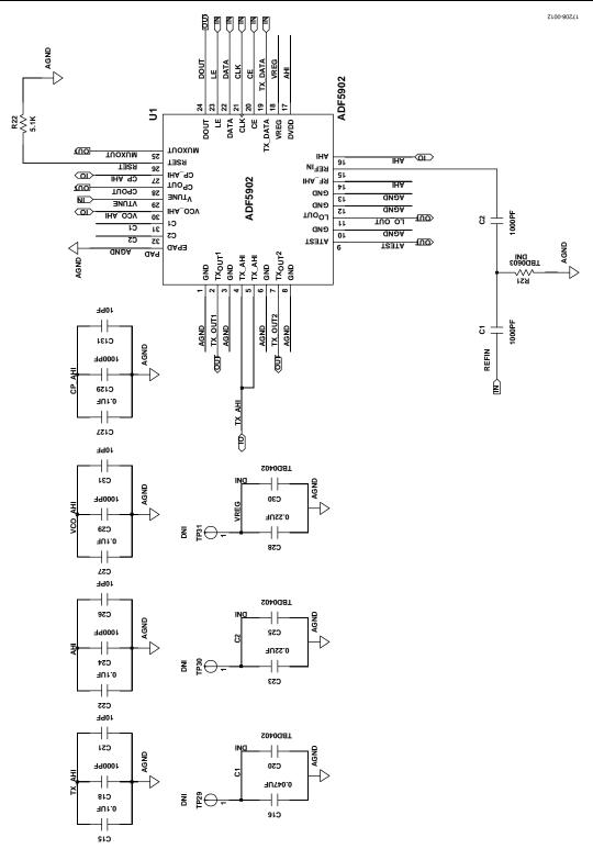
Figure 12. EV-ADF5902SD1Z Evaluation Board Schematic (Page 7)
