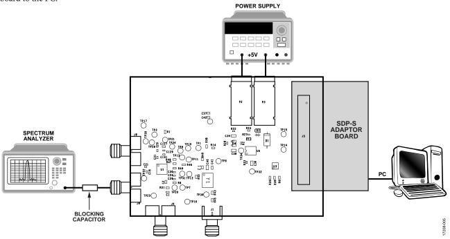
Figure 2. Typical EV-ADF5902SD1Z Evaluation Board Setup
