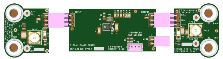
Figure 2. Proper Measurement Equipment Setup (Use SMA connectors for Measuring Input or Output Ripple)
