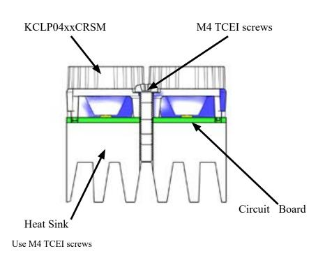
• M4: Maximum tightening torque  $\sim 0.8/1.2~\text{Nm}$
