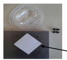
As shown in the photo, the test paper sheet is completely dry after disassembling the system.
