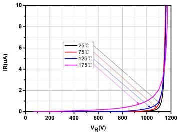
Fig.2-Typical Reverse Characteristics
