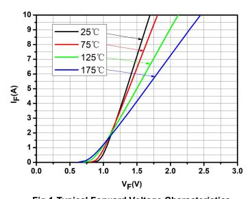
Fig.1-Typical Forward Voltage Characteristics
