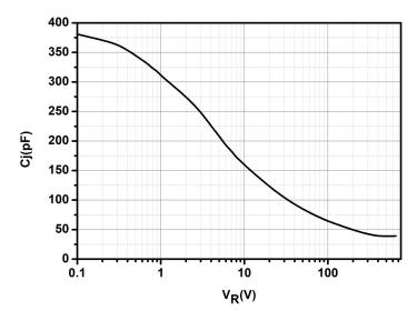
Fig.3-Capacitance vs. Reverse Voltage
