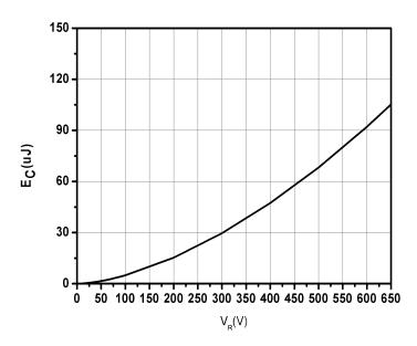
Fig.7-Capacitance Stored Energy
