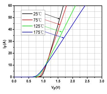
Fig.1-Typical Forward Voltage Characteristics
