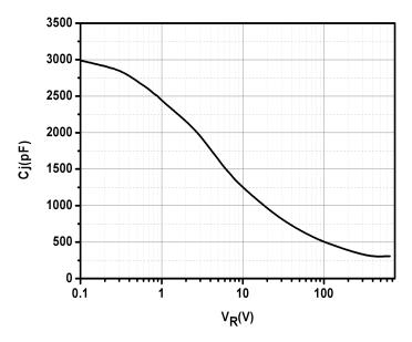
Fig.3-Capacitance vs. Reverse Voltage
