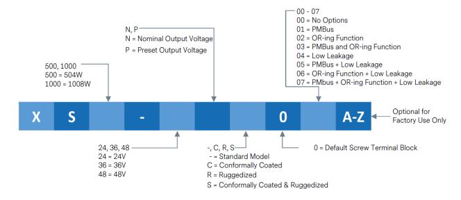
**Example 1:** XS1000-24N-000 = Xsolo 1000 W, 24 V, output with no options **Example 2:** XS1000-24N-003 = Xsolo 1000 W, 24 V, output with PMBus and OR-ing function
