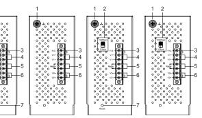
1.Grounding Screw 2.100 BASE-F(X)/1000 BASE(X) 3.Relay Output 1 with current carrying capacity
